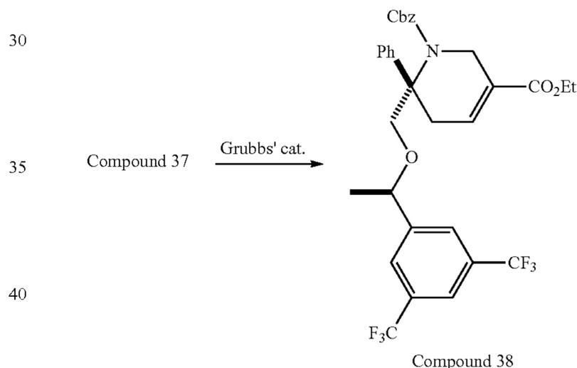
To a solution of Compound 37 (2.46 g, 3.71 mmol, 1 equiv) in anhydrous CH<sub>2</sub>Cl<sub>2</sub> (50 ml) under N<sub>2</sub> was added Grubbs' catalyst (327 mg, 0.385 mmol, 0.1 equiv). The resulting brown solution was heated at 40-45° C. overnight. The solvent was then removed and the residue was purified on a silica gel column to afford Compound 38 (2.1 g, 89%).
