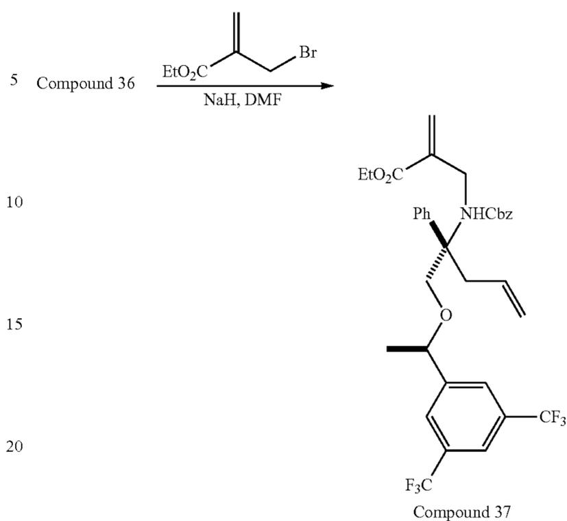
Compound 37 (50% yield) was prepared using similar procedure as for Compound 32 using Compound 36 in place of Compound 17.
