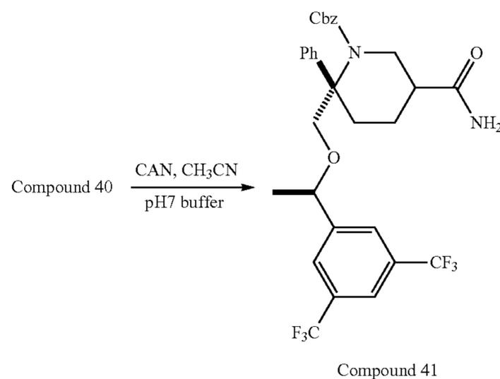
A solution of Compound 40 (1 g, 1.38 mmol, 1 equiv) in  $\text{CH}_3\text{CN}$  (10 ml) and pH7 buffer (3 ml) was treated with ammonium cerium(IV) nitrate (2.17 g, 3.96 mmol, 2.9 equiv) at RT for 2 h. Aqueous work-up gave the crude product which was purified by silica gel column to give Compound 41 (760 mg, 91%).
