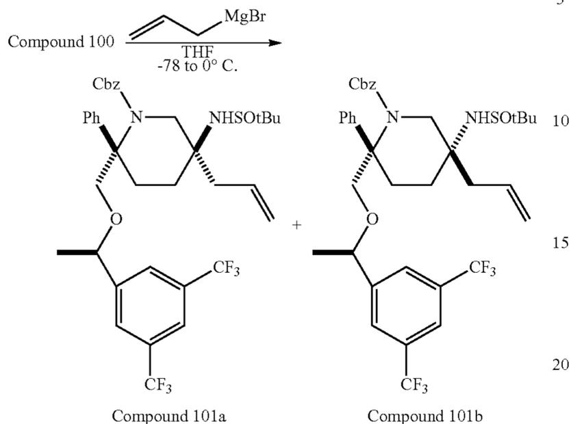
Following a procedure similar to Example 11, Step 3, Compound 100 was converted to sulfinamide Compounds 101a and 101b.
