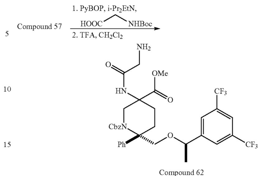
Compound 57 was converted to Compound 62 (72% yield over two steps) using the PyBOP coupling followed by TFA deprotection procedures as described in the preparation of Example 62 from Compound 55 but using Compound 57 (1 equiv.) in place of ammonia and NH-Boc-glycine (2 equiv.) in place of Compound 55.
