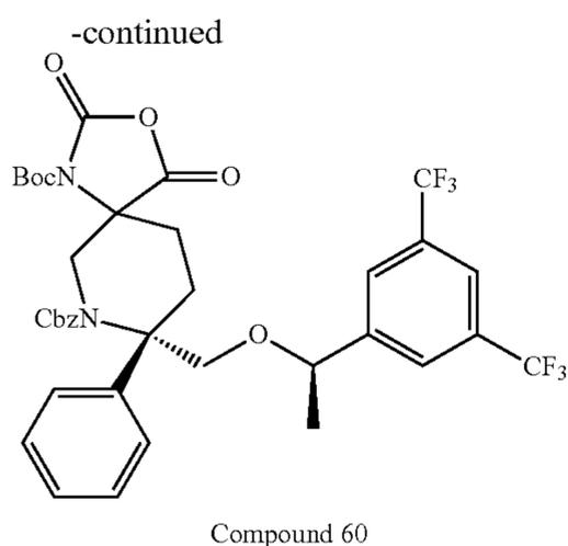
To a solution of crude Compound 53 (19 g) in  $\text{CH}_2\text{Cl}_2$  (300 ml) at RT, DIEA (15 ml, 0.087 mol) was added, followed by triphosgene (4.34 g, 0.015 mol). The mixture was stirred at RT for 18 h and was filtered through a pad of silica. Solvents were removed in vacuum to give crude Compound 60 as yellow oil which was used in the next reaction without further purifications.
