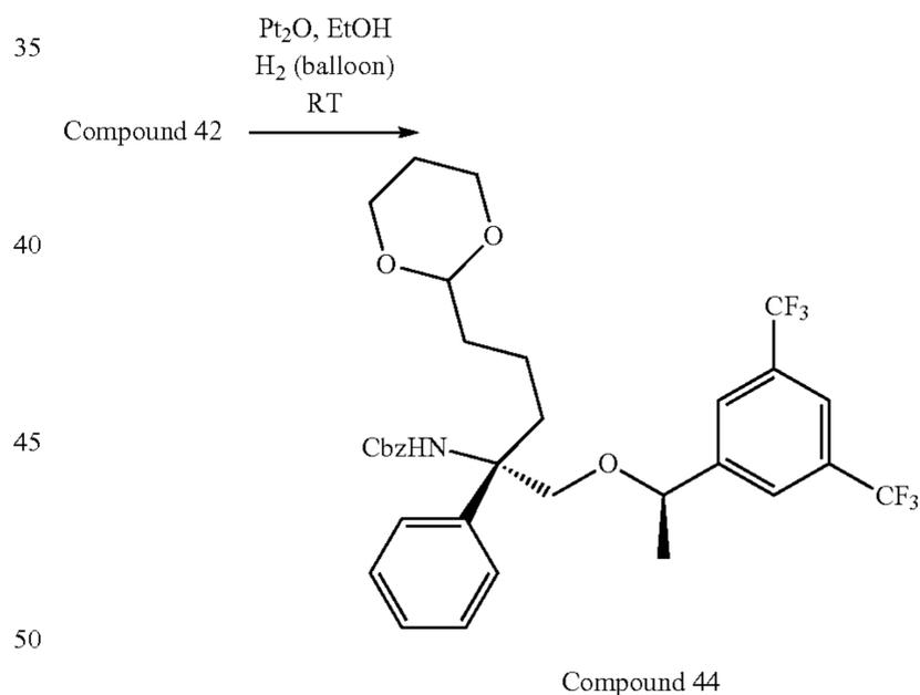
A suspension of alkene Compound 42 (40.5 g, 64 mmol, 1 equiv.) and  $\text{PtO}_2$  (1.44 g, 6.4 mmol, 0.1 equiv.) in EtOH (400 ml) were stirred under a  $\text{H}_2$  balloon at  $23^\circ\text{C}$ . for 24 h. Another batch of  $\text{PtO}_2$  (1.44 g, 6.4 mmol, 0.1 equiv) was added and the mixture was stirred for another 24 h at  $23^\circ\text{C}$ . The catalyst was filtered via a pad of Celite. This solution of alkane Compound 44 was used in the next step without further purification.
