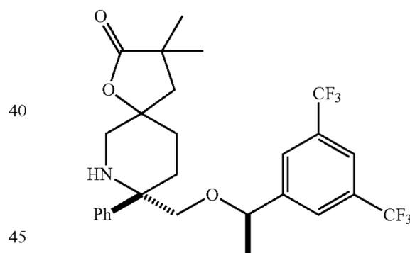
Example 59 (75%) was prepared from Example 57b in a manner similar to that used to prepare Example 58 from Example 57a. Electrospray MS [M+1]<sup>+</sup>=530.1.
