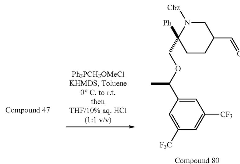
Compound 80 (72% yield) was prepared by similar procedure as for Compound 23 using Compound 47 in place of Compound 3.
