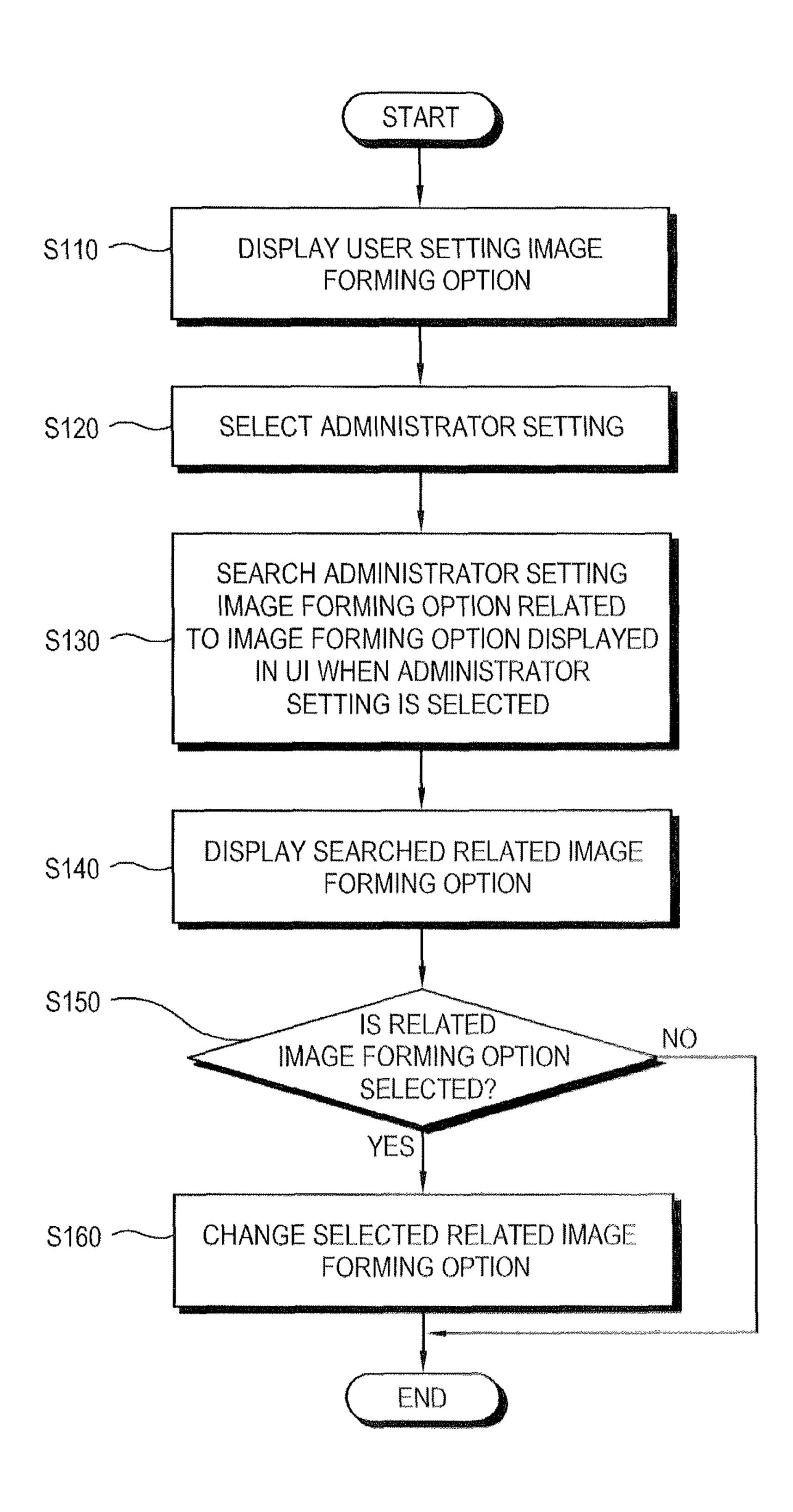
IMAGE FORMING APPARATUS AND IMAGE FORMING OPTION SETTING METHOD THEREOF TO DISPLAY AN ADMINISTRATOR SETTING OPTION HAVING A CORRELATION WITH THE DISPLAYED USER SETTING OPTION ACCORDING TO THE SELECTED ADMINISTRATOR SETTING
