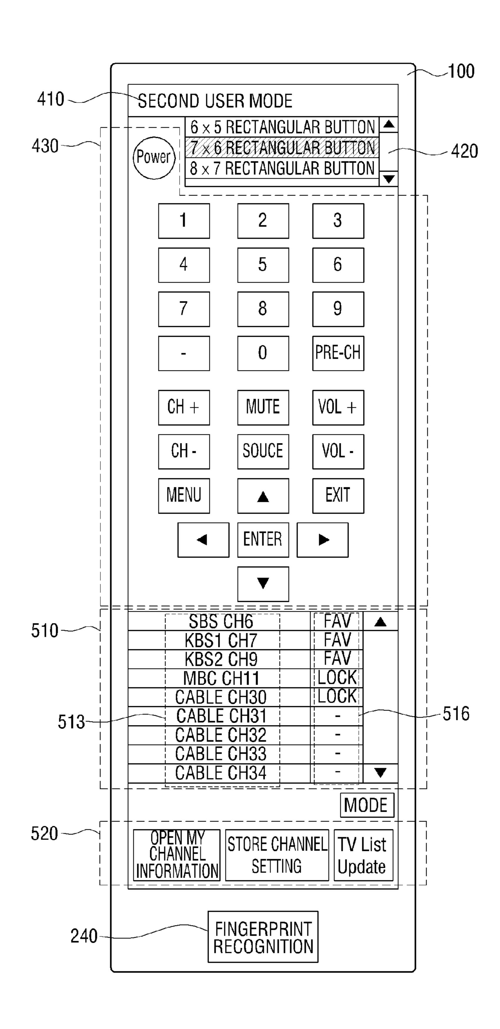
FIG. 6 \_100 410 ~ THIRD USER MODE 420 8 x 7 RECTANGULAR BUTTON PRE-CH ENTER 440 MODE CH LIST | RETURN | TOOLS **INFO** CC CH LIST INTERNET RETURN MODE | TOOLS || **INFO** CC MEDIA CONTRNT GUIDE HDMI FINGERPRINT RECOGNITION
