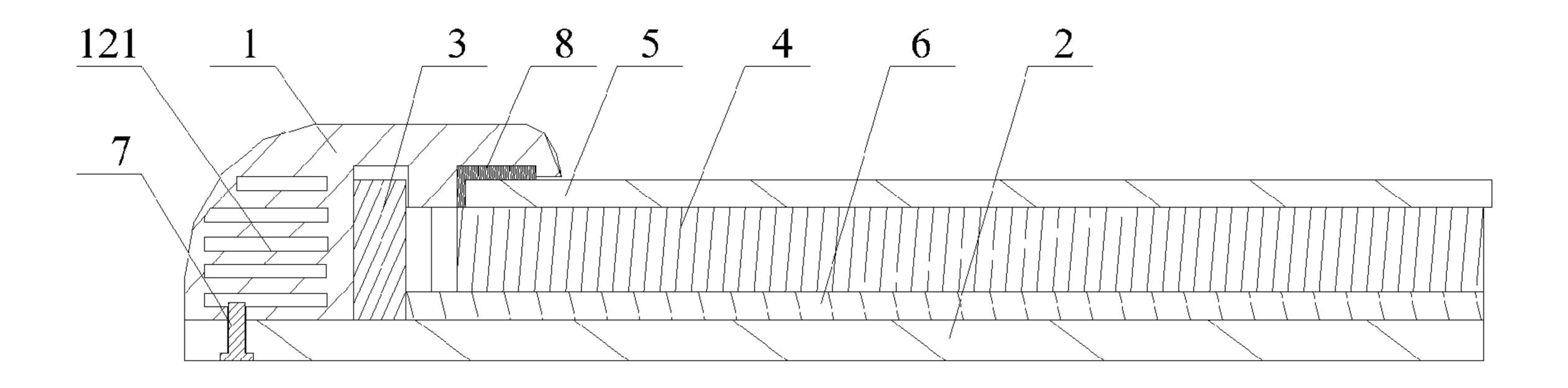
machine of the liquid crystal display, which simplifies the heat transmission way, reduces the thermal contact resistance and increases the effective heat-dissipation area of the front casing Thereby, the heat caused by the LED light source can be synchronously transmitted to the front casing and to the back casing. Besides, the utility model installs a fin heat-dissipation structure on the front casing corresponding to the back of the LED light source, which can improve the heat-
