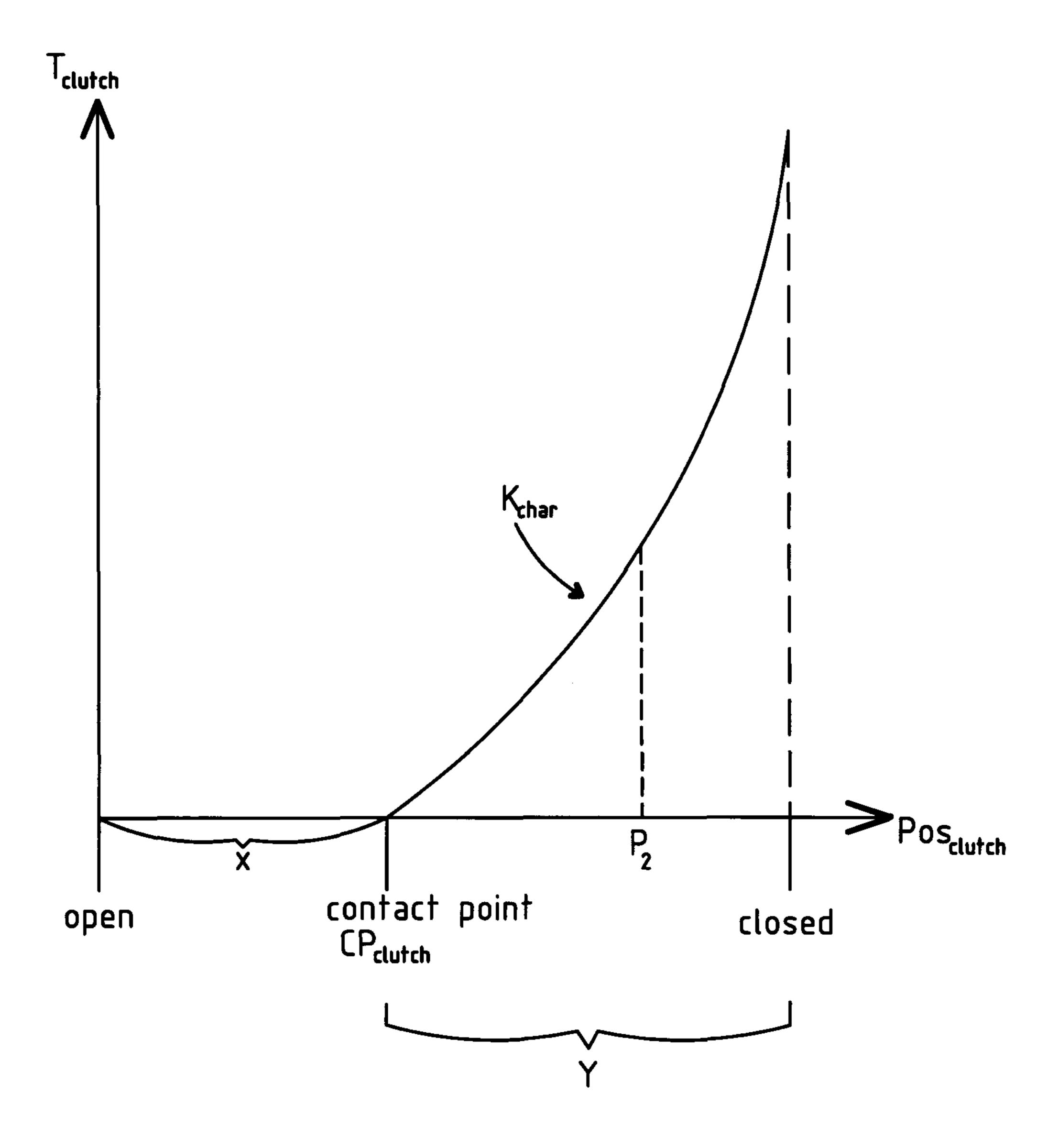
open clutch to first position at initial speed
