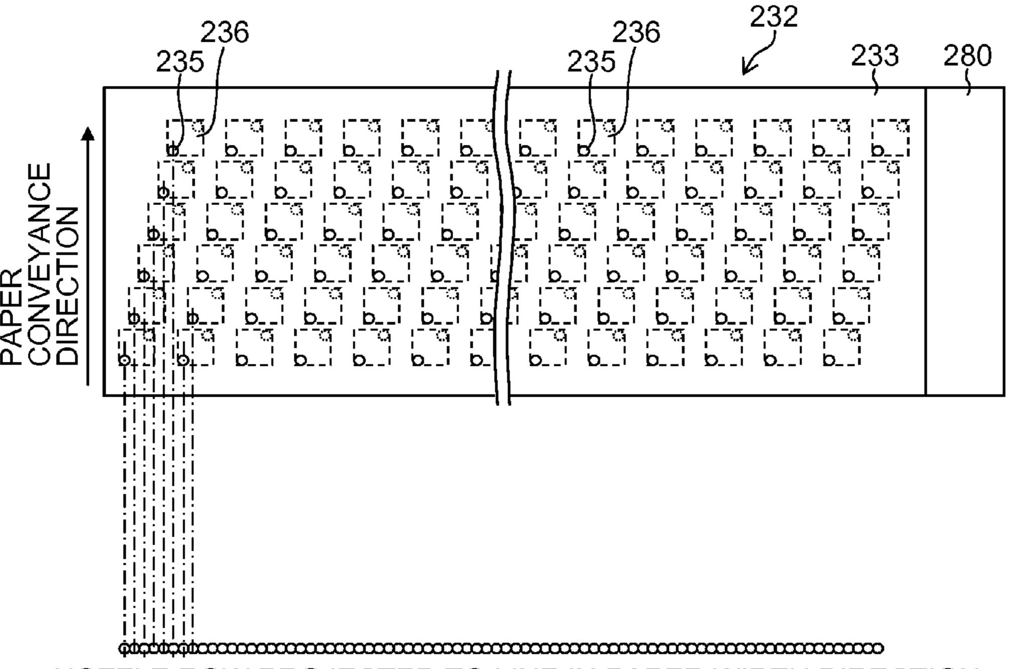
NOZZLE ROW PROJECTED TO LINE IN PAPER WIDTH DIRECTION PERPENDICULAR TO PAPER CONVEYANCE DIRECTION
