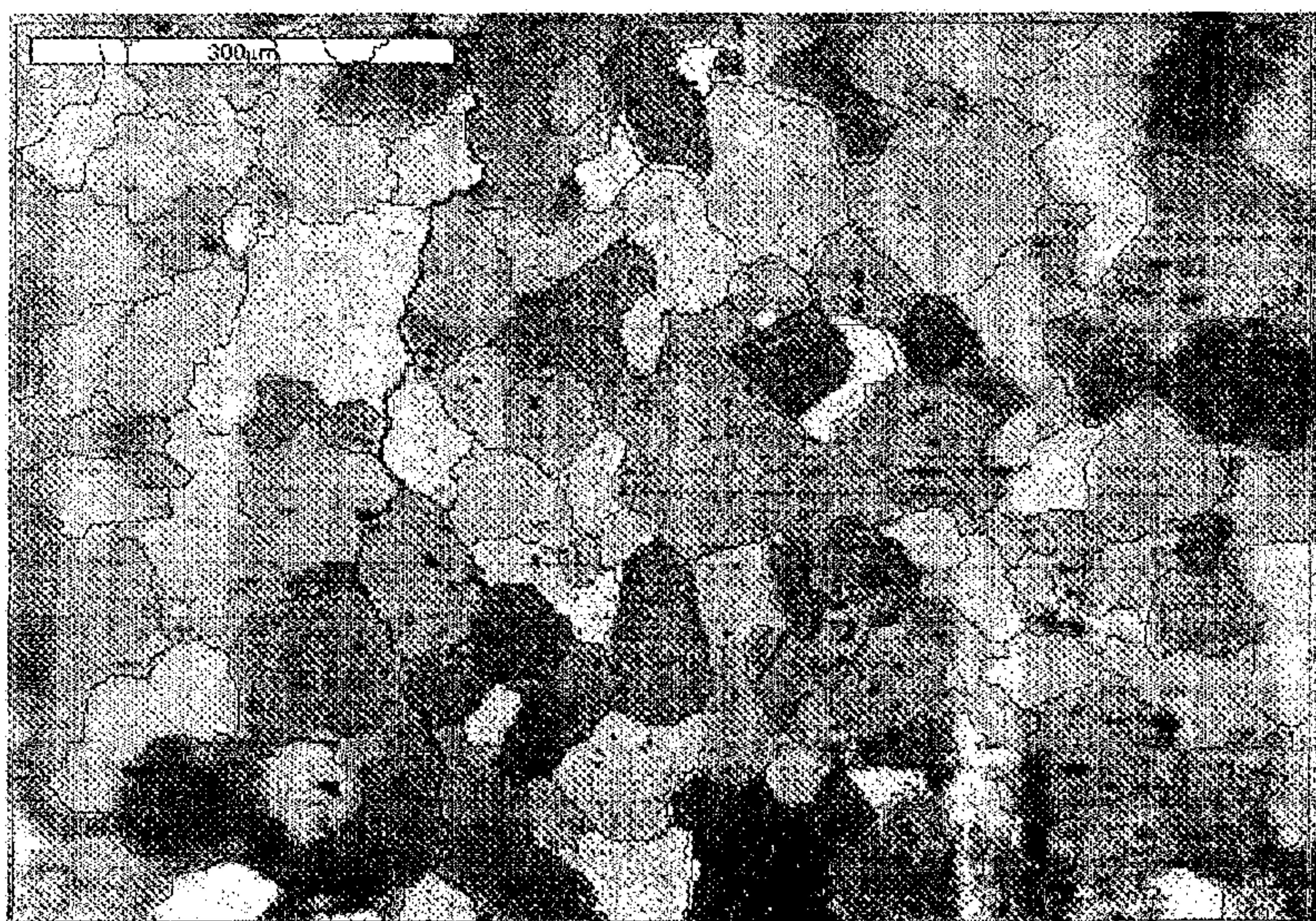
Fig. 2 : Grain boundaries overlaid on SEM micrograph
