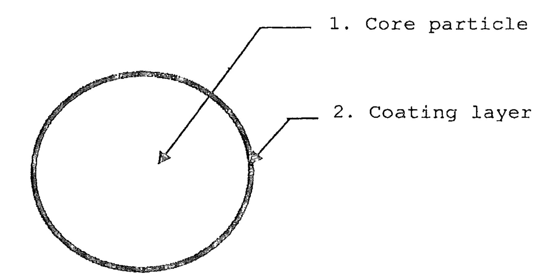
NICKEL OXIDE POWDER MATERIAL FOR SOLID OXIDE TYPE FUEL CELL AND METHOD FOR PRODUCING THE SAME, AND ANODE MATERIAL, ANODE AND SOLID OXIDE TYPE FUEL CELL USING THE SAME
