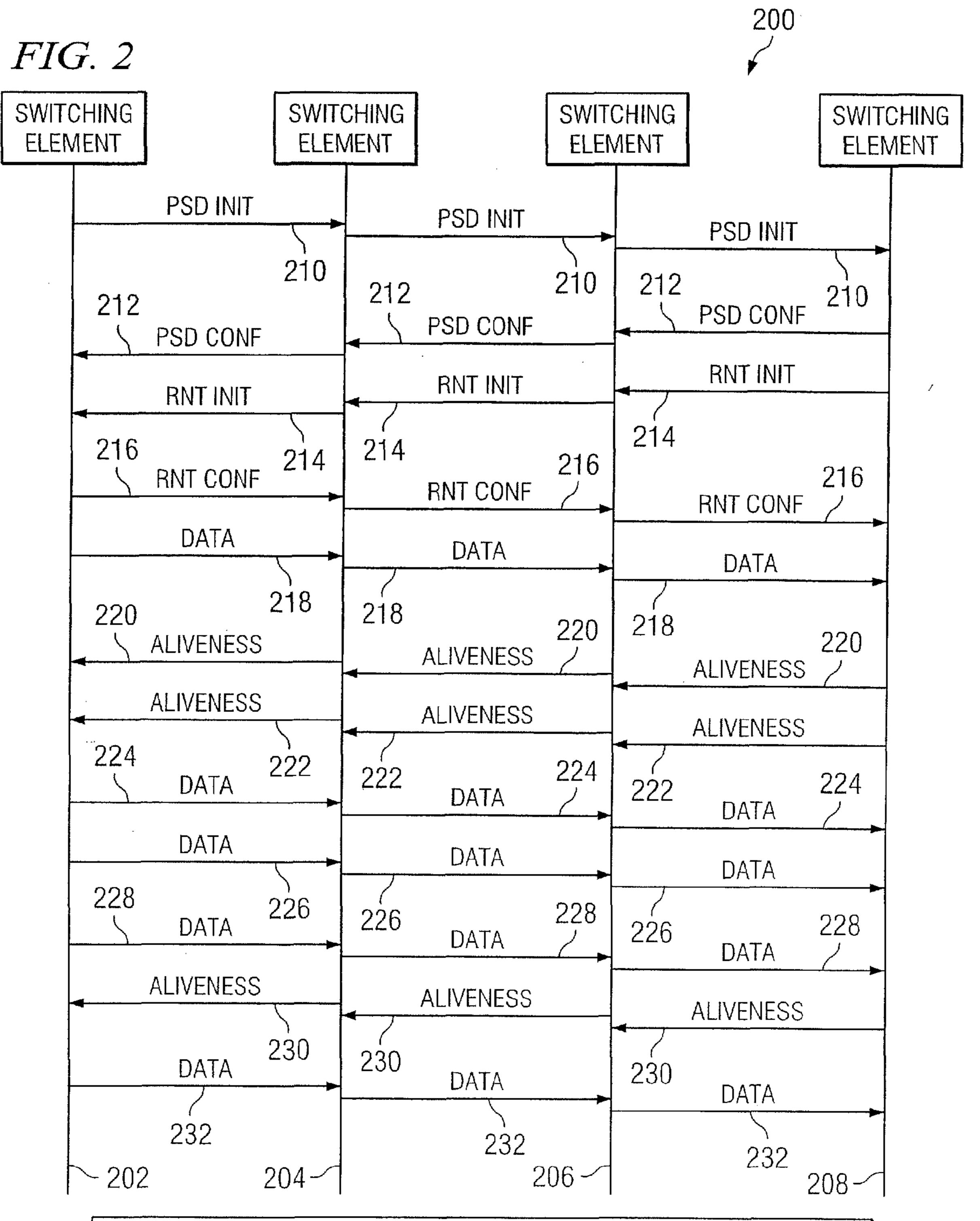
PSD=PROTECTION SWITCH DOMAIN (ESTABLISHMENT OF THE WORKING AND PROTECTION PATH: IDENTIFICATION OF SWITCHING ELEMENTS)
