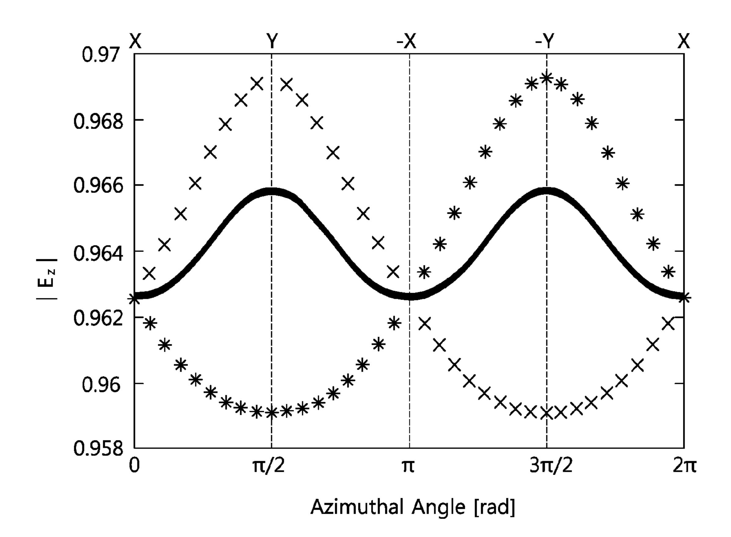
X : dipole field caused by coupling hole
