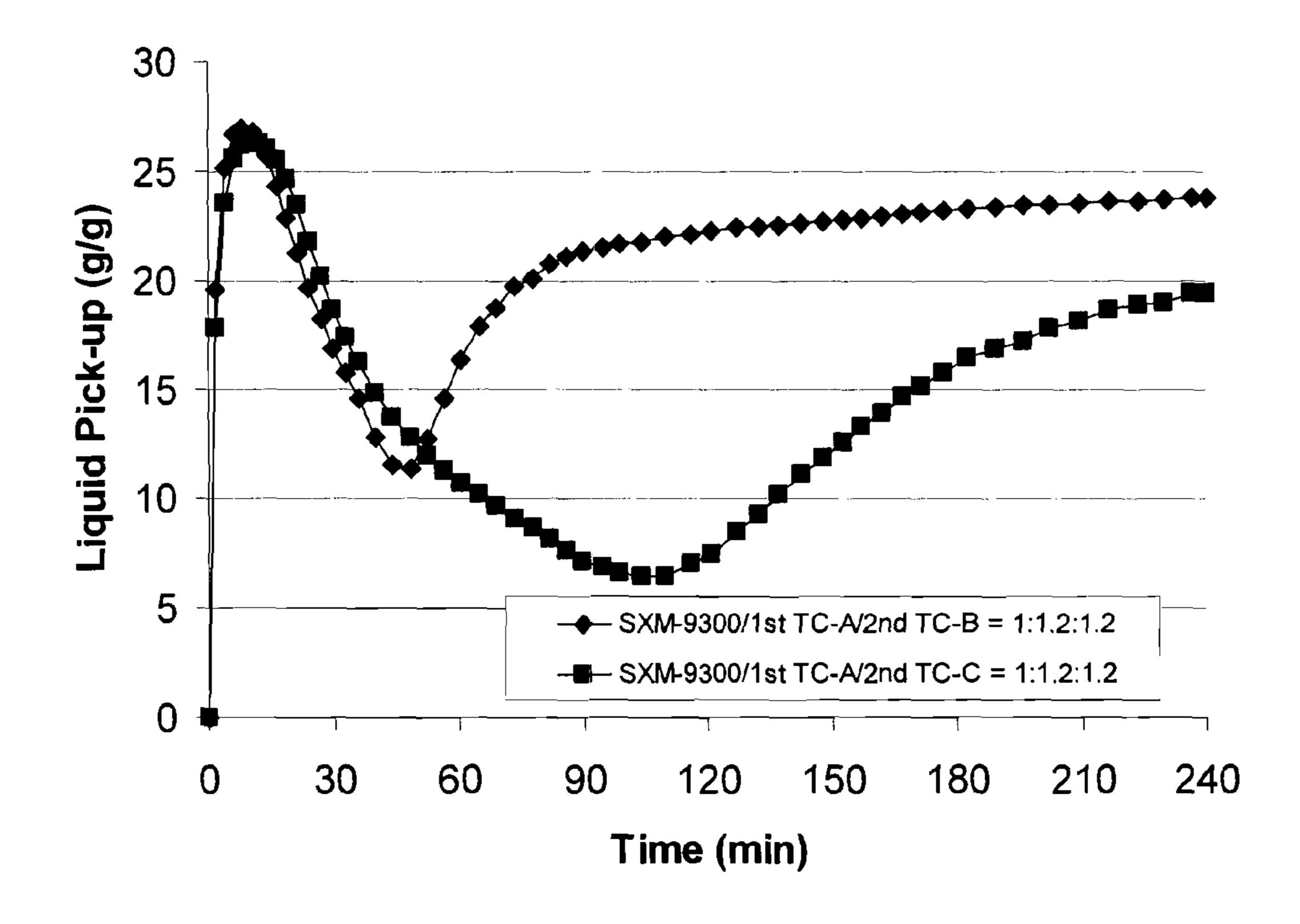
FIG 8. Swell/deswell/reswell curves for superabsorbent composition SAP-B and with triggering compositions 1<sup>st</sup> TC-A and 2<sup>nd</sup> TC-B
