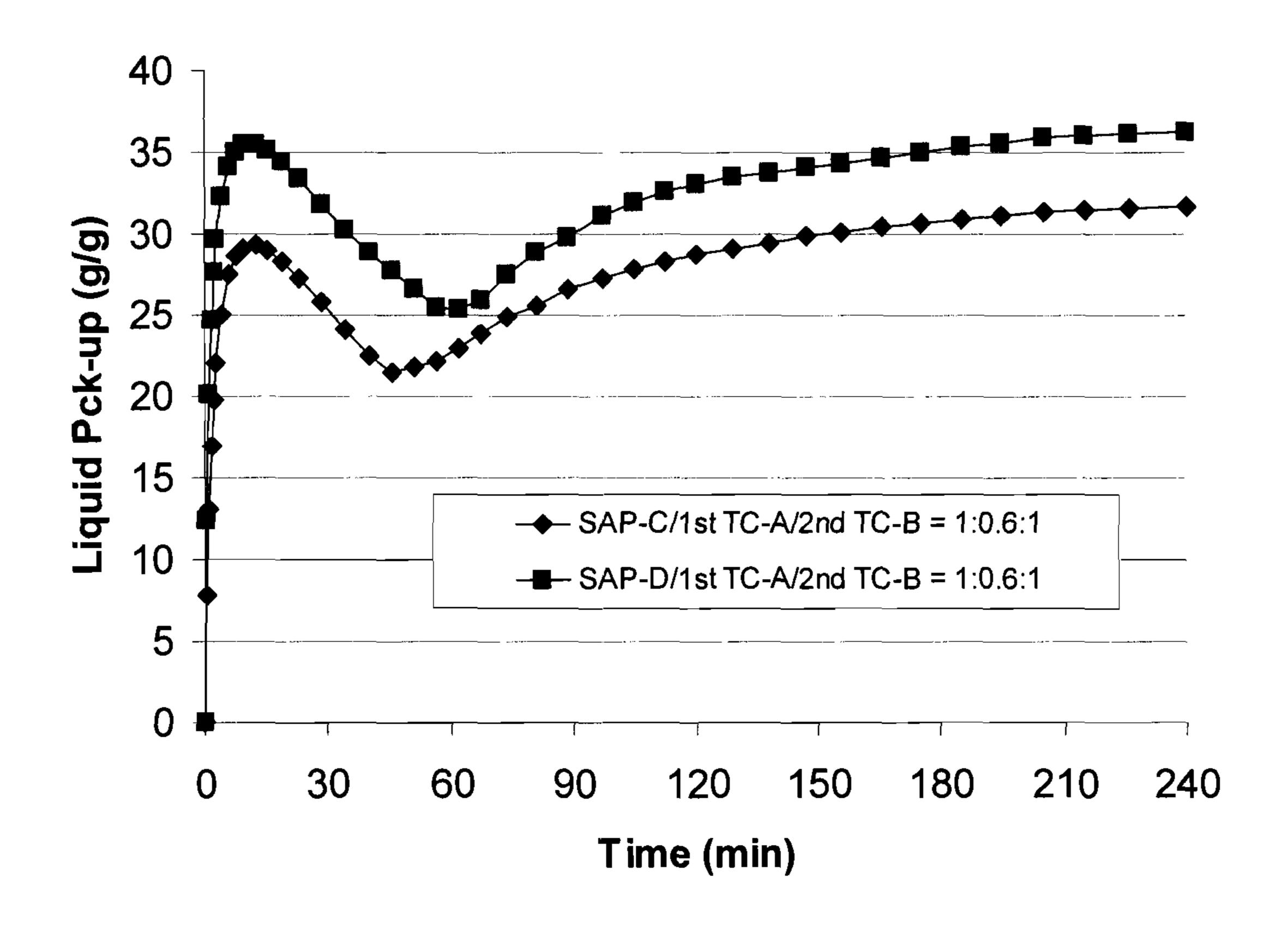
FIG 10. Swell/deswell/reswell curves for a specific commercial SAP product and with triggering compositions 1<sup>st</sup> TC-C and 2<sup>nd</sup> TC-A
