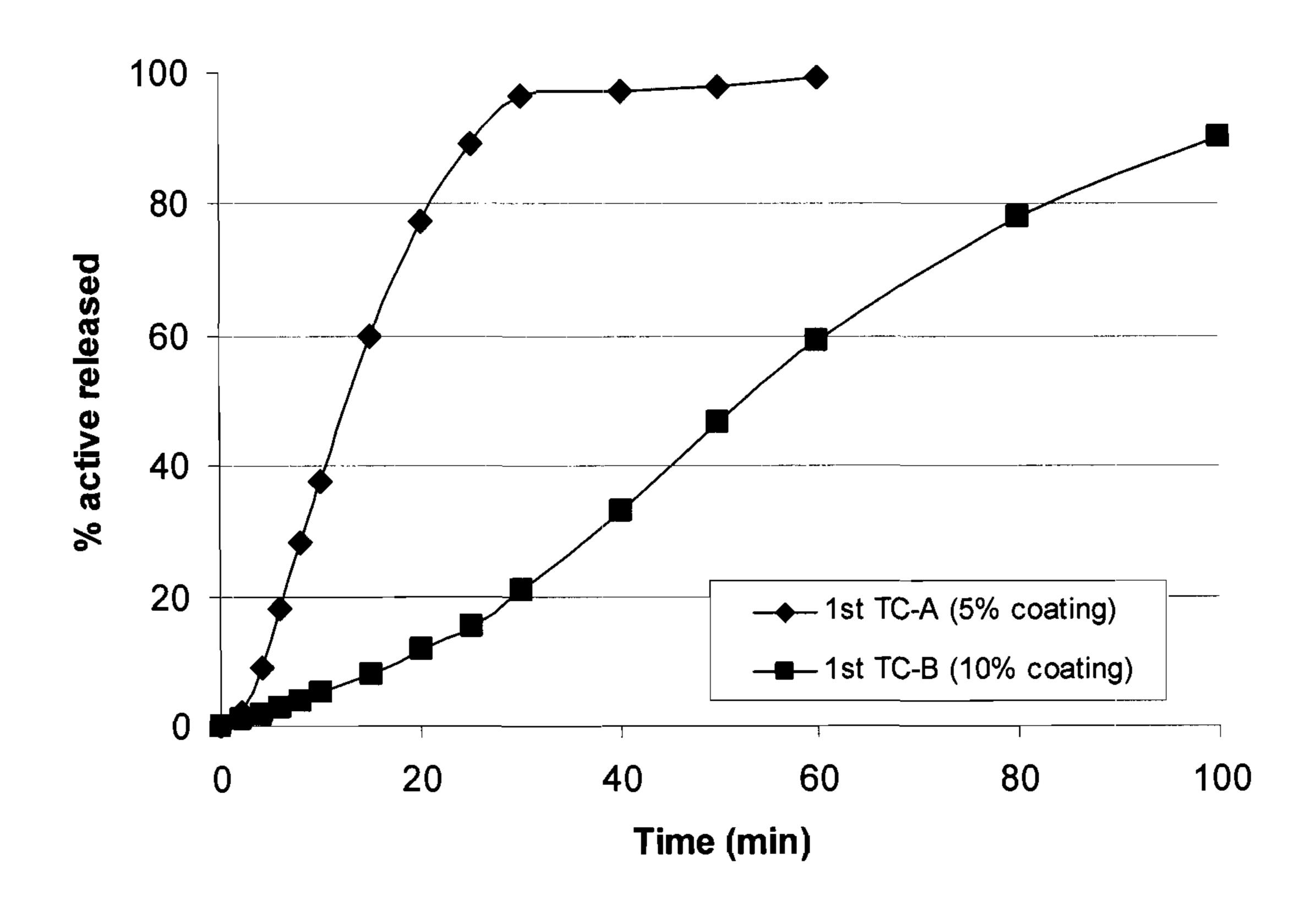
FIG 2. Release profiles of poly(meth)acrylate coated calcium formate
