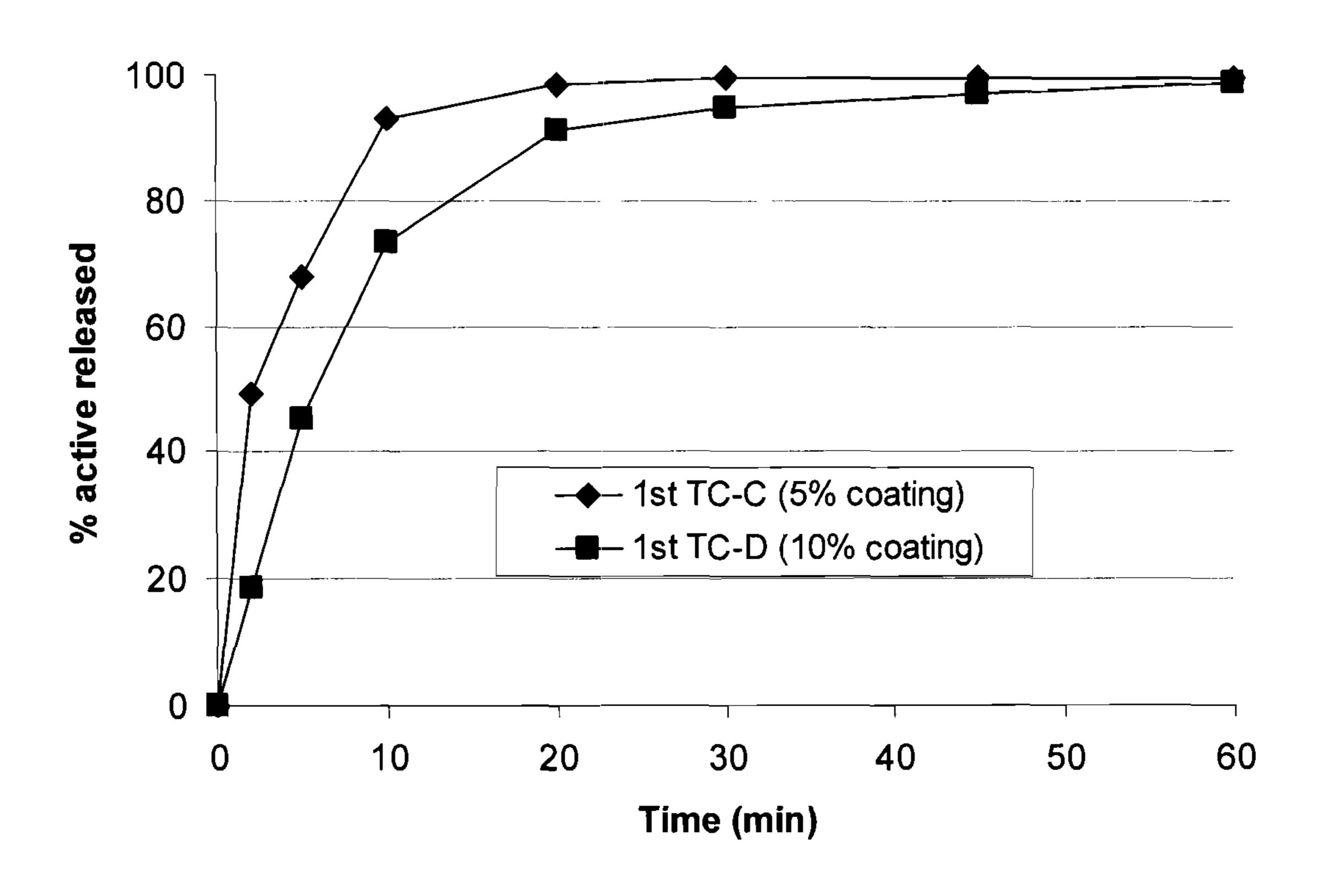
FIG 3. Release profiles of cellulose acetate or cellulose acetate/ethyl cellulose coated calcium formate
