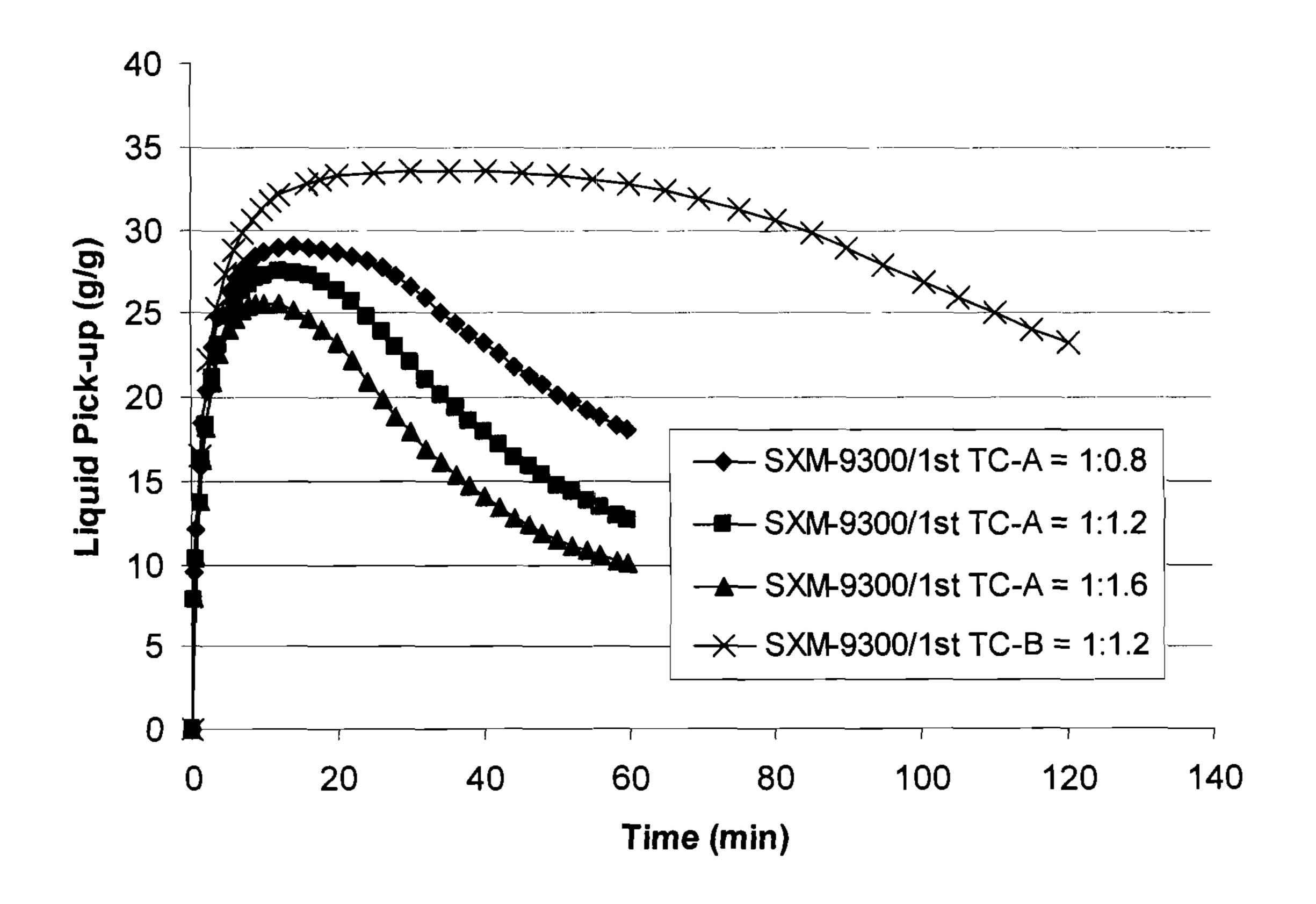
FIG 7. Swell/deswell/reswell curves for SXM-9300 and with various blends of 1<sup>st</sup> and 2<sup>nd</sup> triggering compositions
