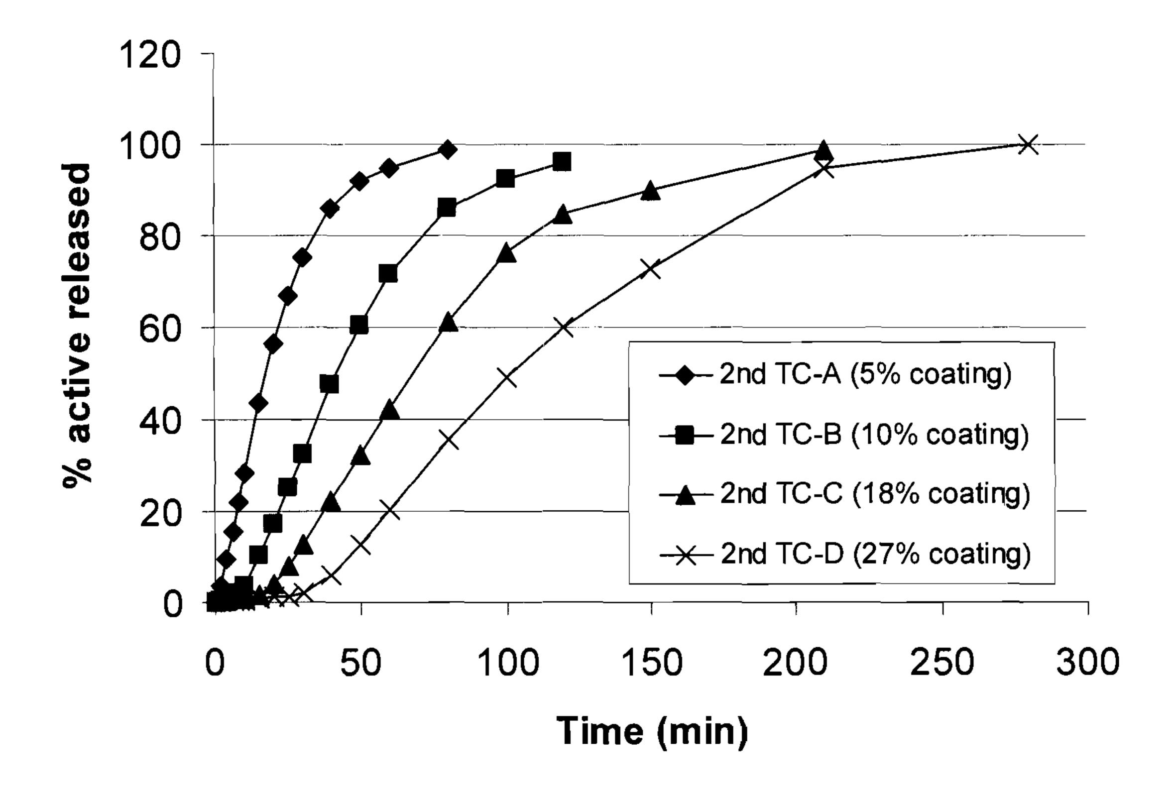
FIG 5. Release profiles of maleated polypropylene coated sodium carbonate
