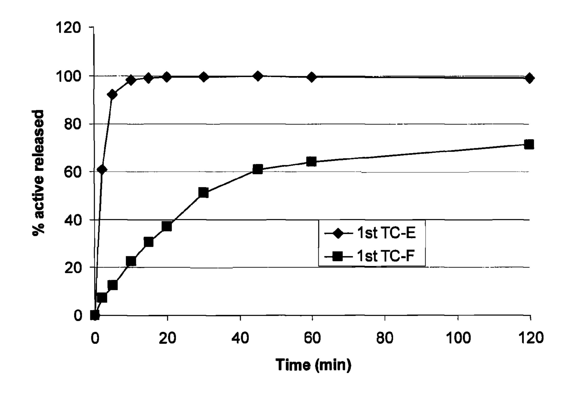
FIG 4. Release profiles of poly(meth)acrylate coated sodium carbonate
