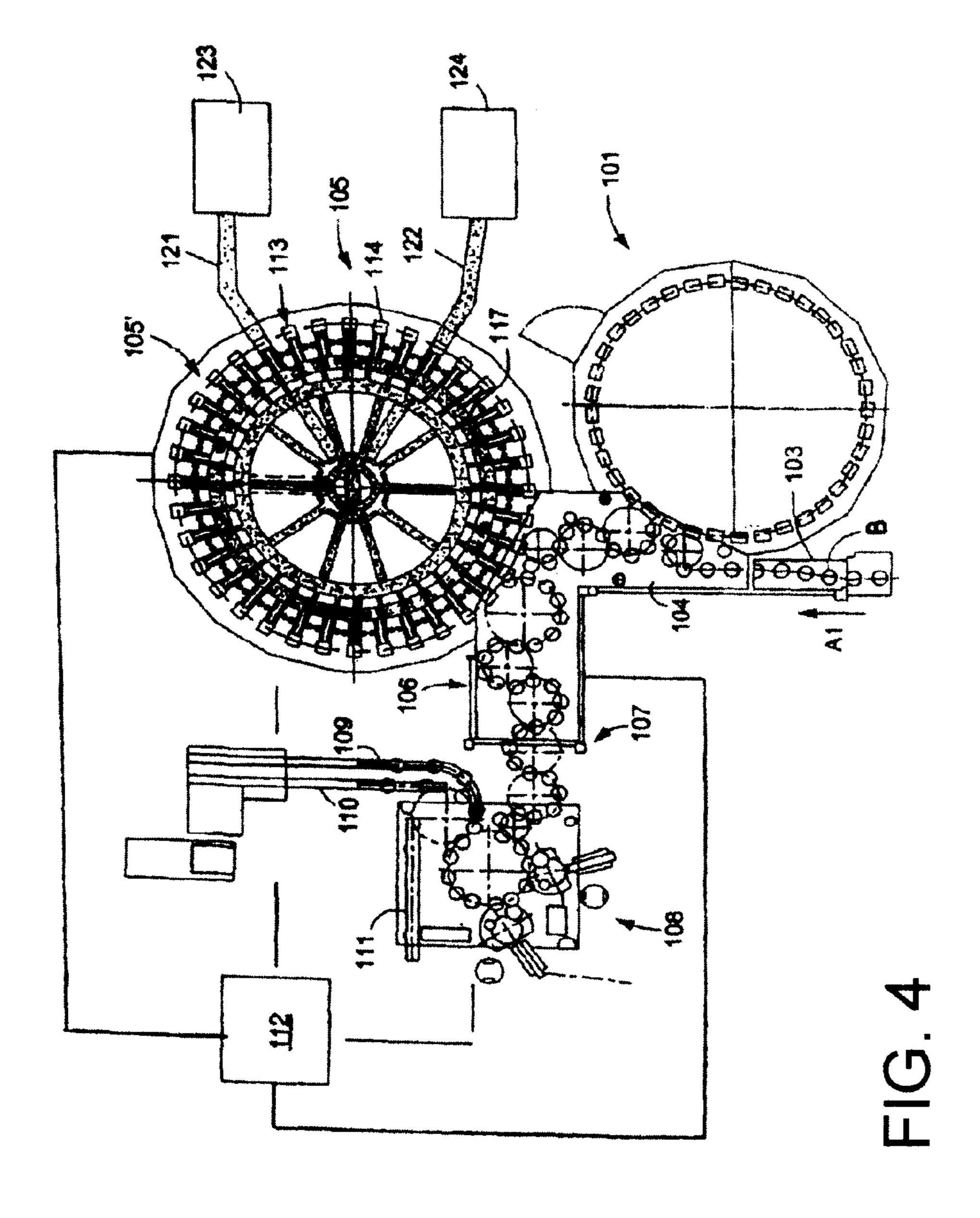
METHOD FOR FILLING BOTTLES OR SIMILAR CONTAINERS WITH AN OXYGEN SENSITIVE EFFERVESCENT LIQUID BEVERAGE FILLING MATERIAL UNDER COUNTERPRESSURE AND FILLING MACHINE FOR THE PERFORMANCE OF THIS METHOD
