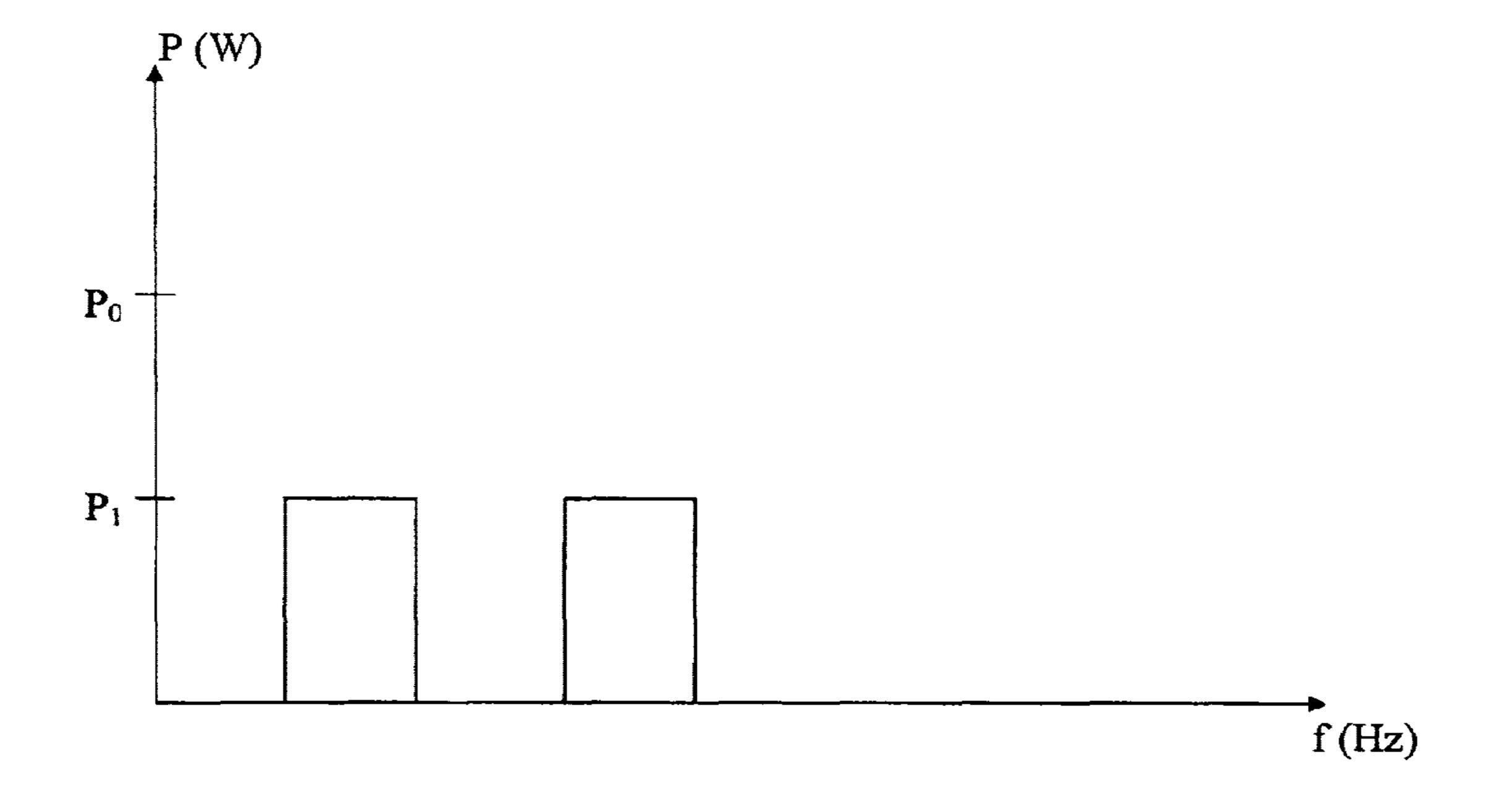
2 Channels @ 6.4 MHz each Modulation = 32 QAM Data Rate = 50 Mbps  $P_{TOTAL} = 2*P_1 = P_0$
