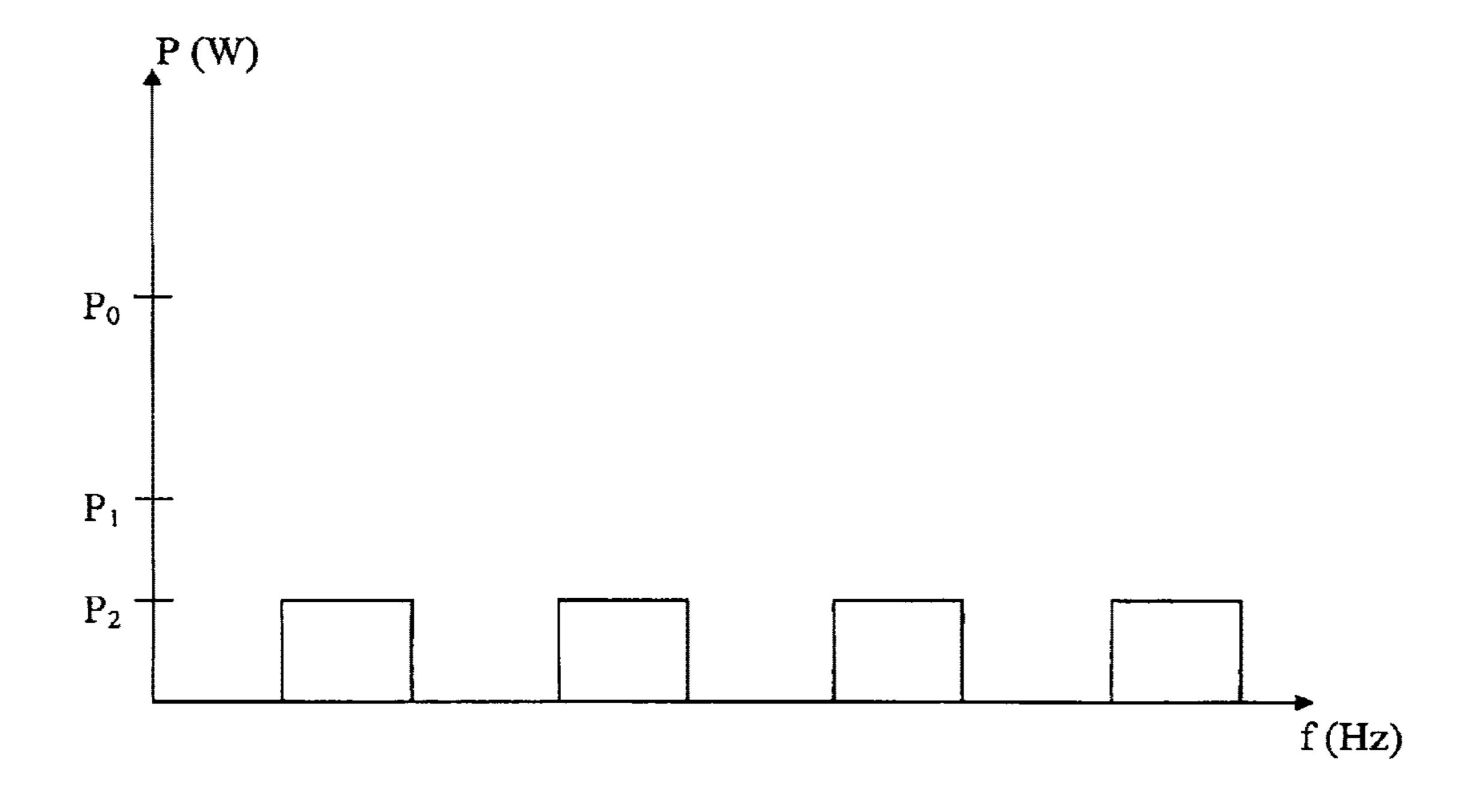
4 Channels @ 6.4 MHz each Modulation = 16 QAM Data Rate = 80 Mbps  $P_{TOTAL} = 4*P_2 = P_0$
