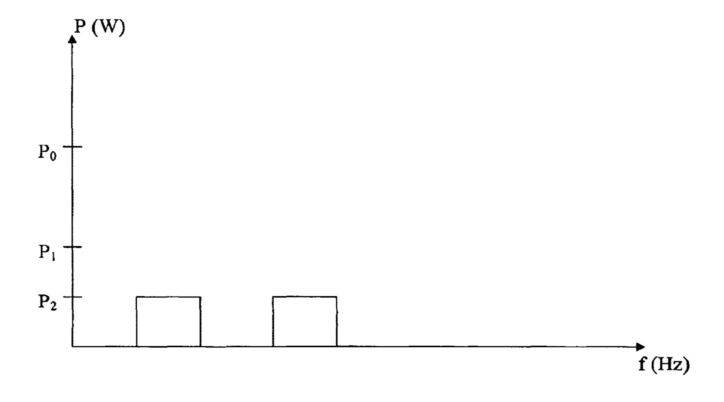
2 Channels @ 6.4 MHz each Modulation = 16 QAM Data Rate = 40 Mbps  $P_{TOTAL} = 2*P_2 = \frac{1}{2} P_0$
