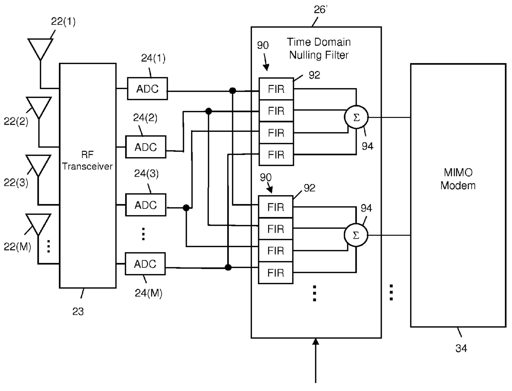
Nulling parameters (coefficients/taps of FIR filters) based on type of interference
