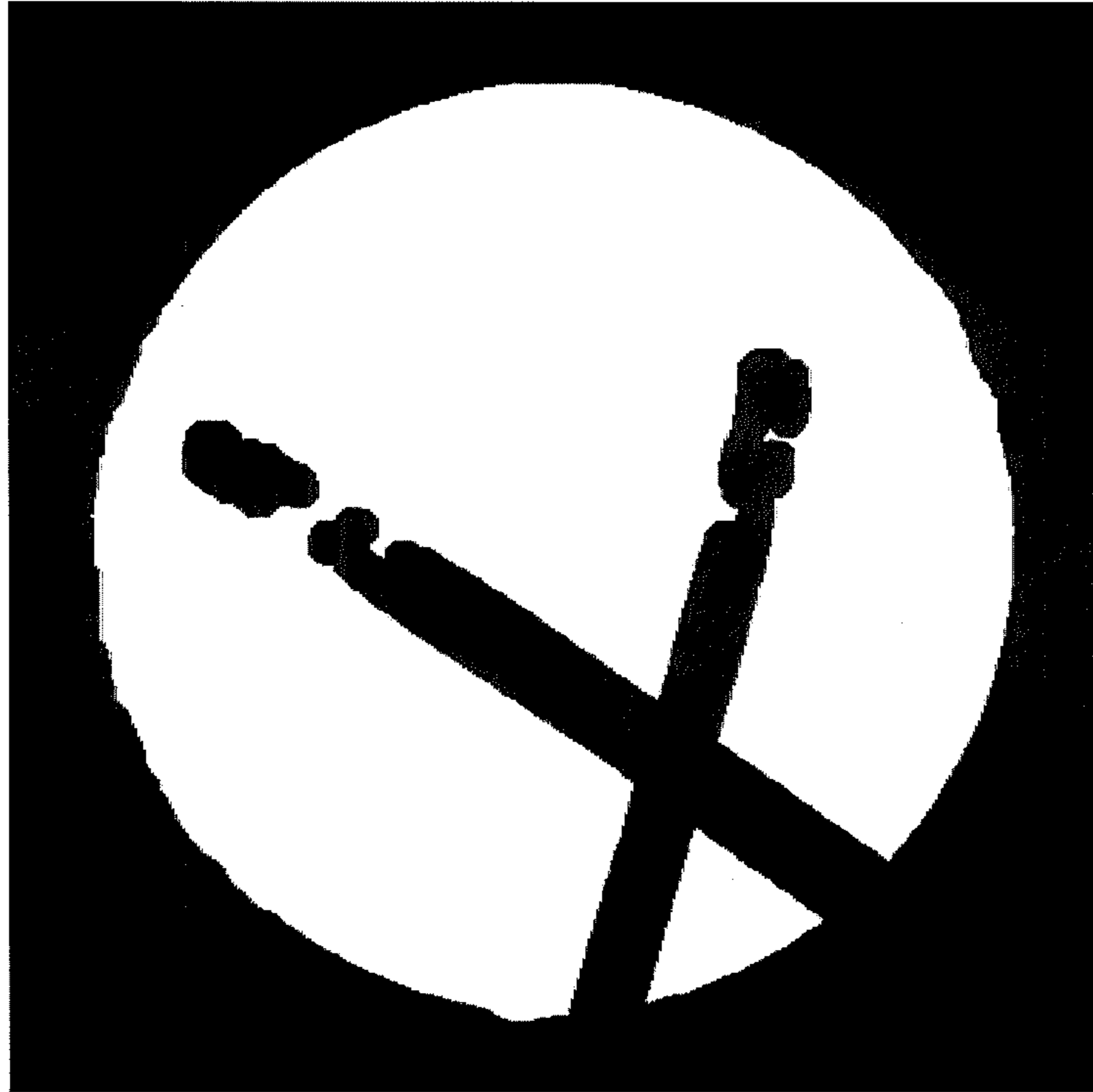
Threshold Mask after Dilation and Erosion
