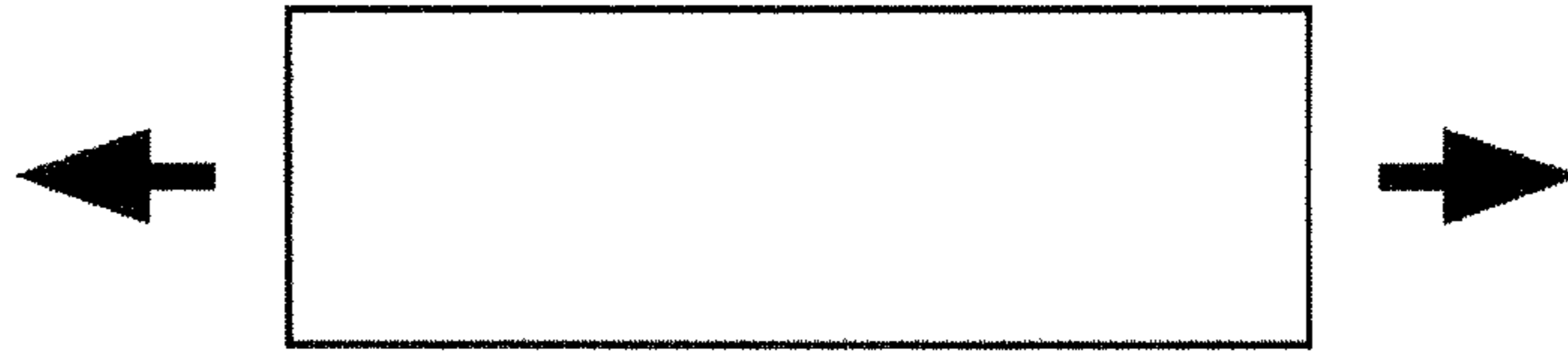
Fig. 6A Tension, Positive Strain
