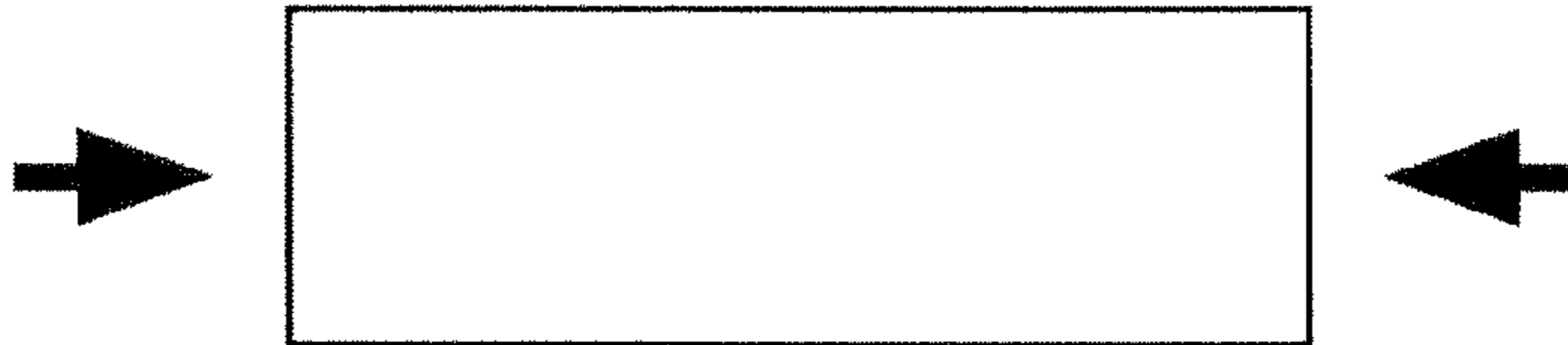
Fig. 6B Compression, Negative Strain
