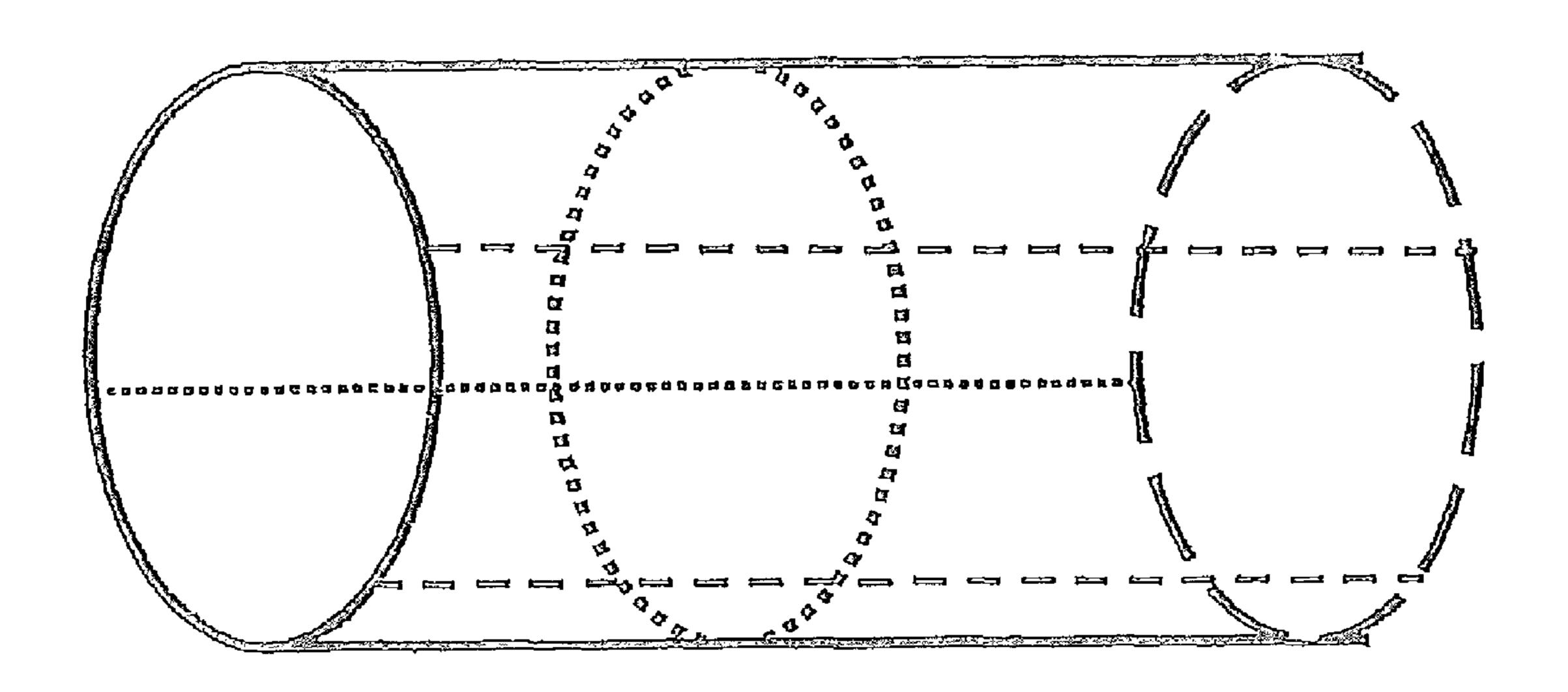
Figure 2. A plug wrap having 60 holes/inch
