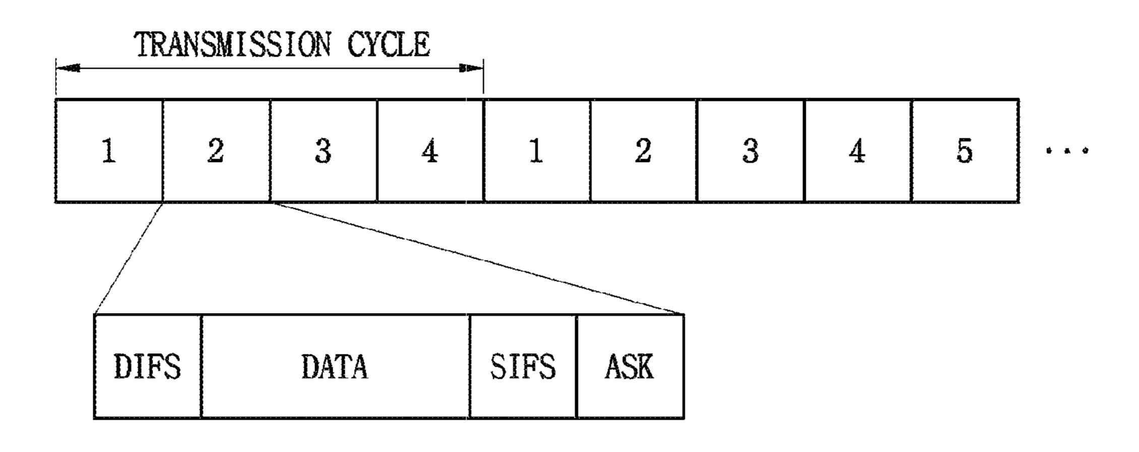
(An Internal Structure of a Transmission Unit When a Conventional Distributed Coordination Function(DCF) is Used)
