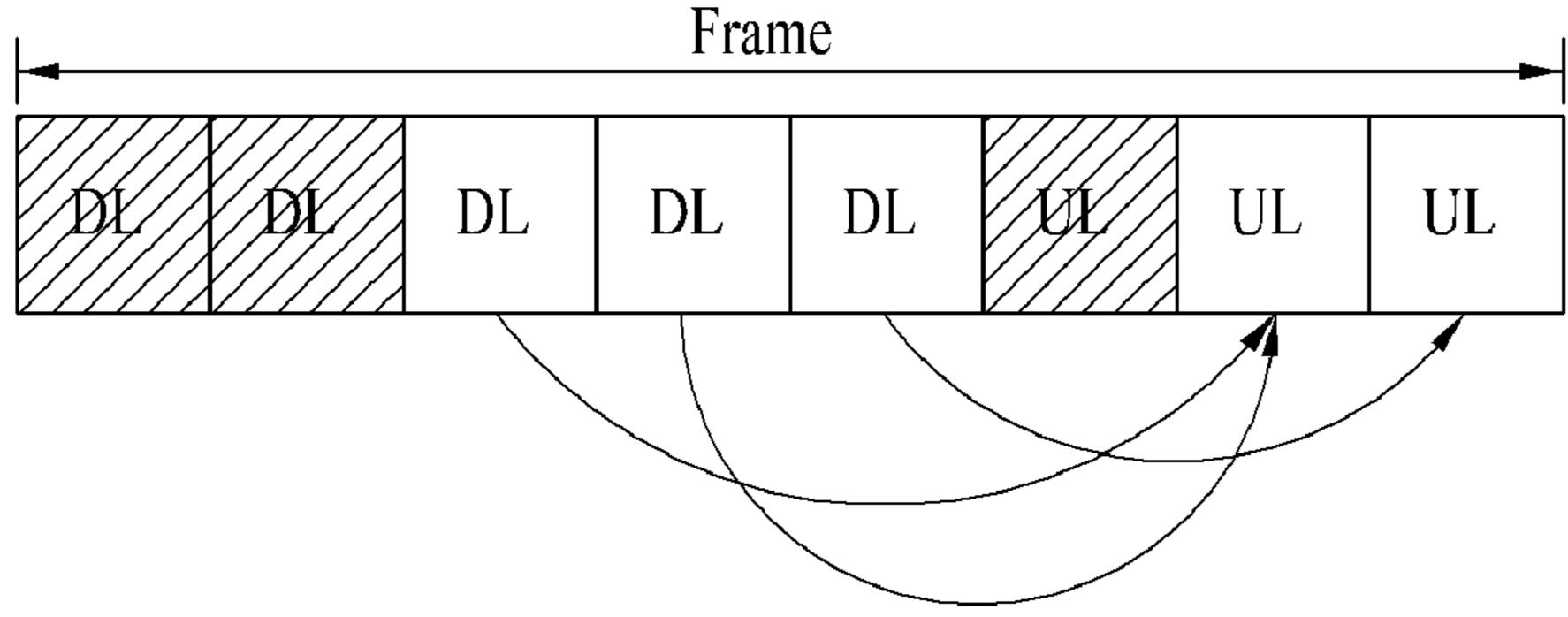
UL ACK timing for DL burst transmission
