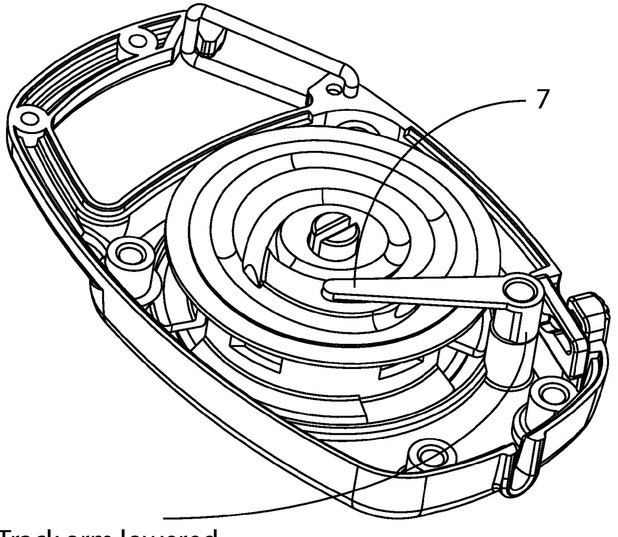
Track arm lowered into no-tension mode
