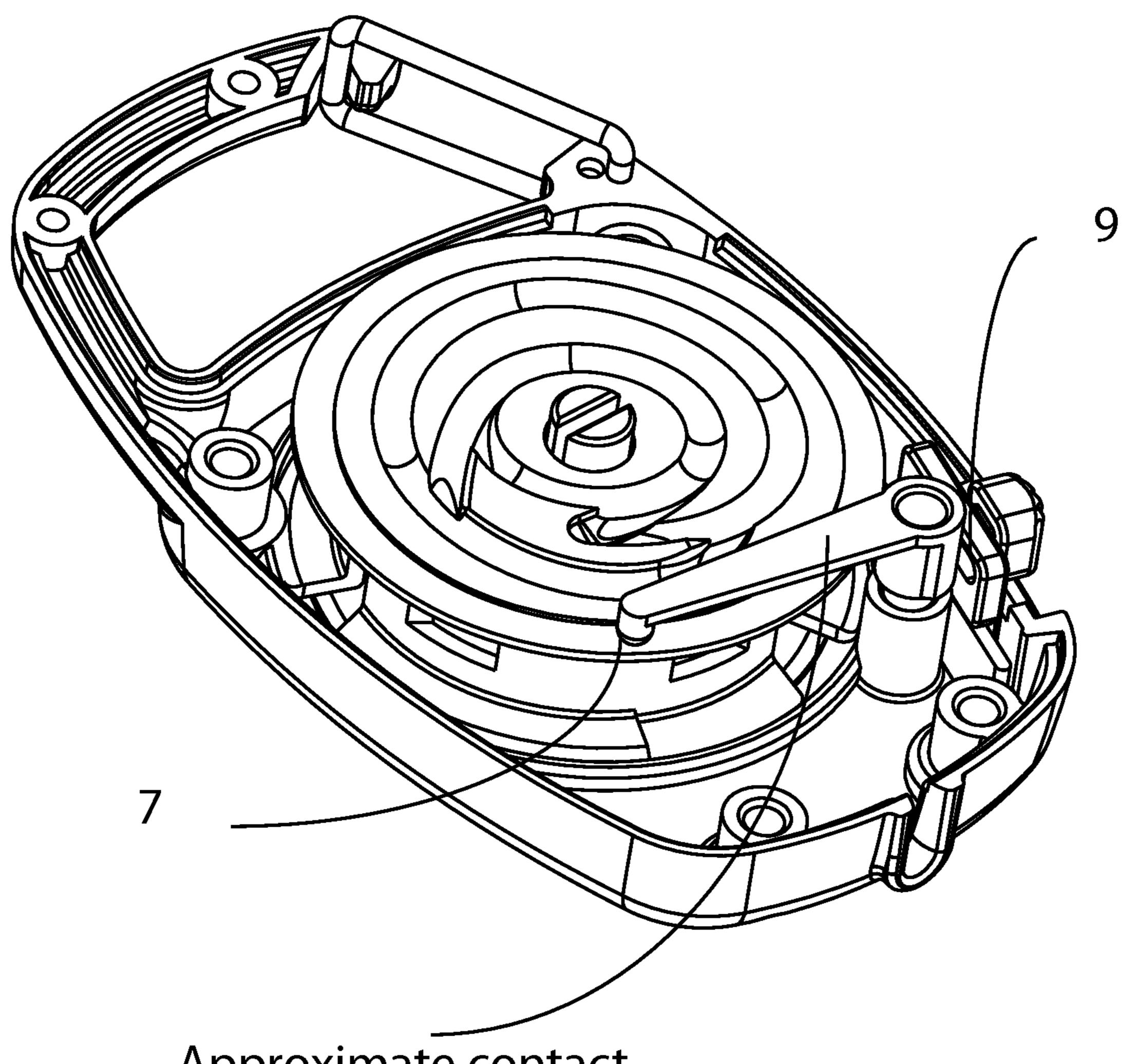
Approximate contact point to lever-rib23 on top half of enclosure
