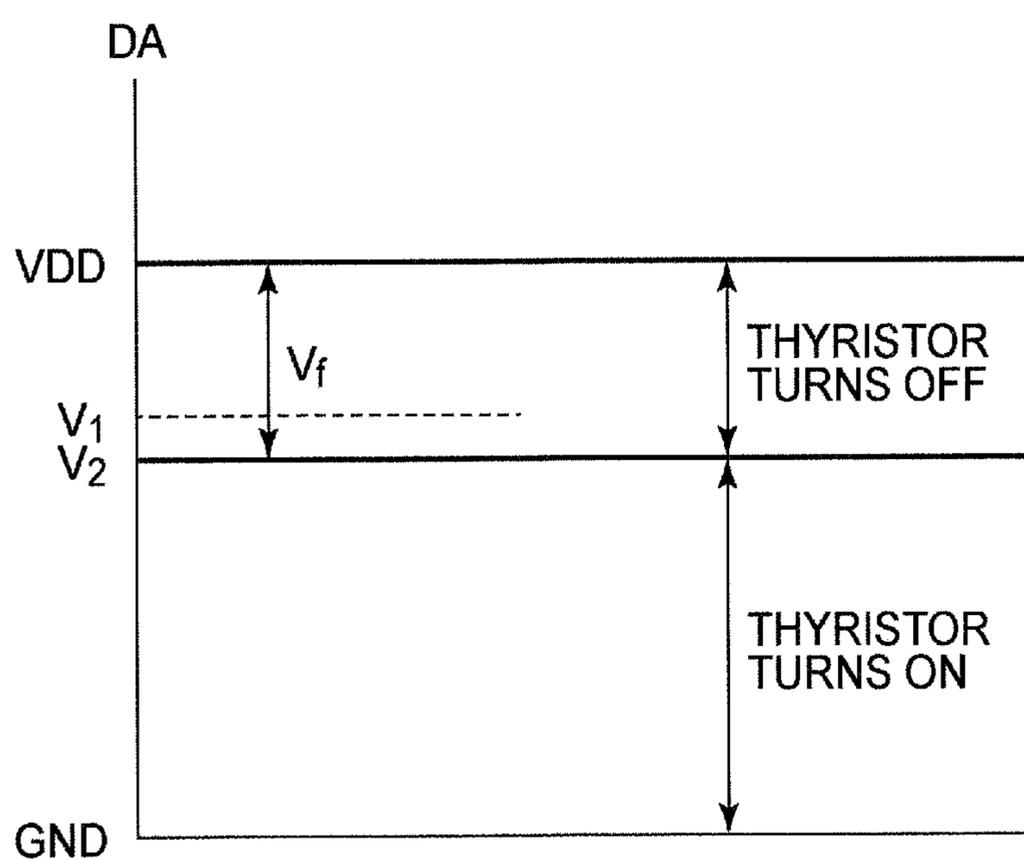
$$V_1 = \frac{R_{65}}{R_{64} + R_{65}} \times V_{DD}$$
