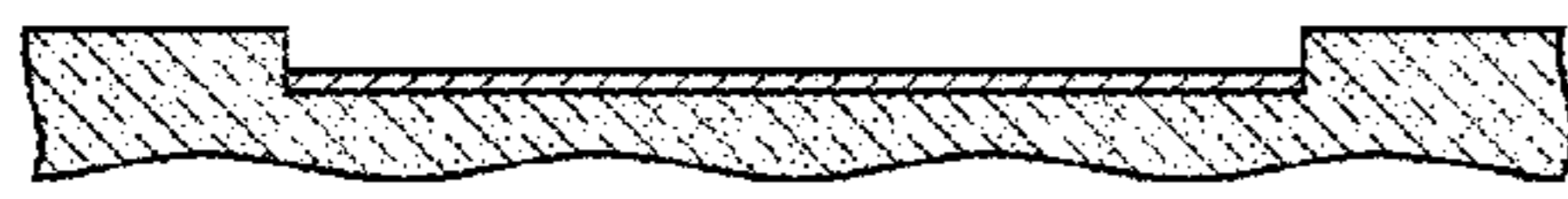
Recess & Shield Metal Layer
