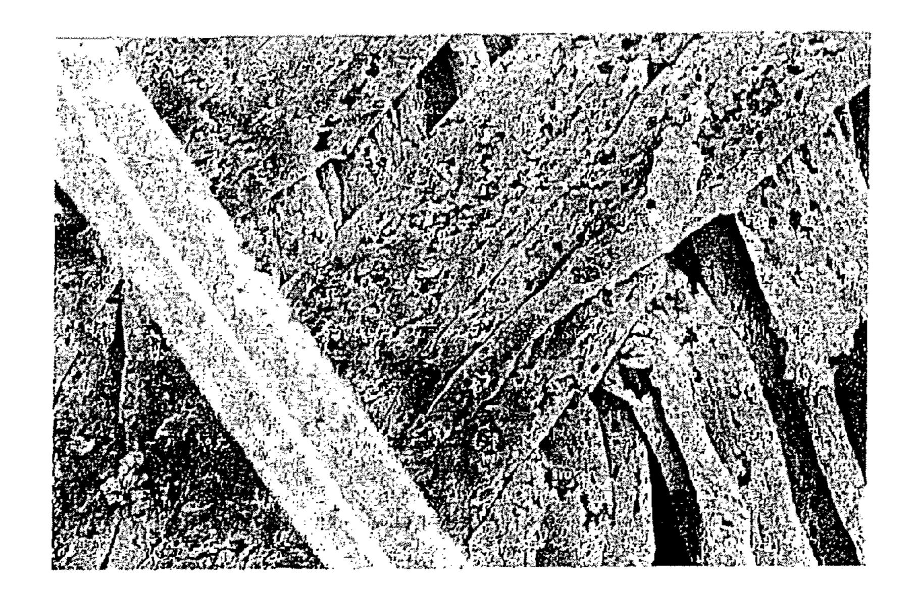
Filaments according to Example 2 after 16 weeks of an outdoor test (SEM, 1,000 times magnification)
