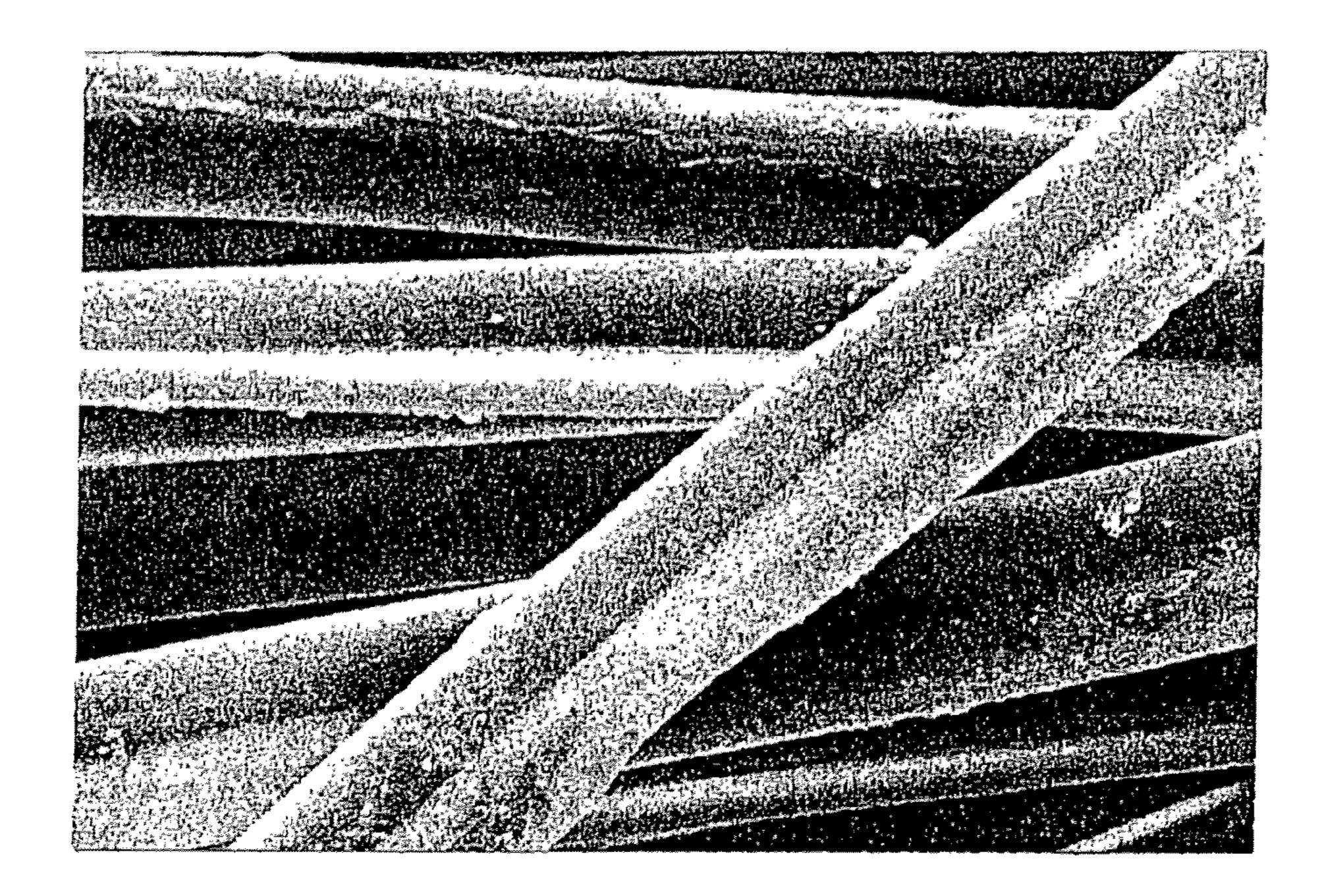
Filaments according to Example 4 after 16 weeks of an outdoor test (SEM, 1,000 times magnification)
