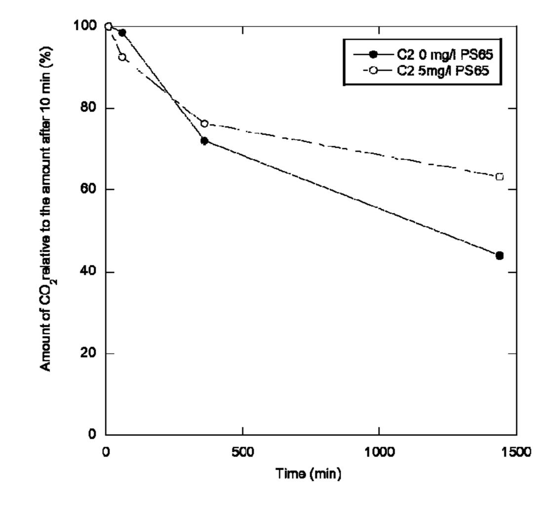
Figure 11: Amount of CO<sub>2</sub> (in % of the amount after 10 min) retained for C2 after removing the cap from the bottle.
