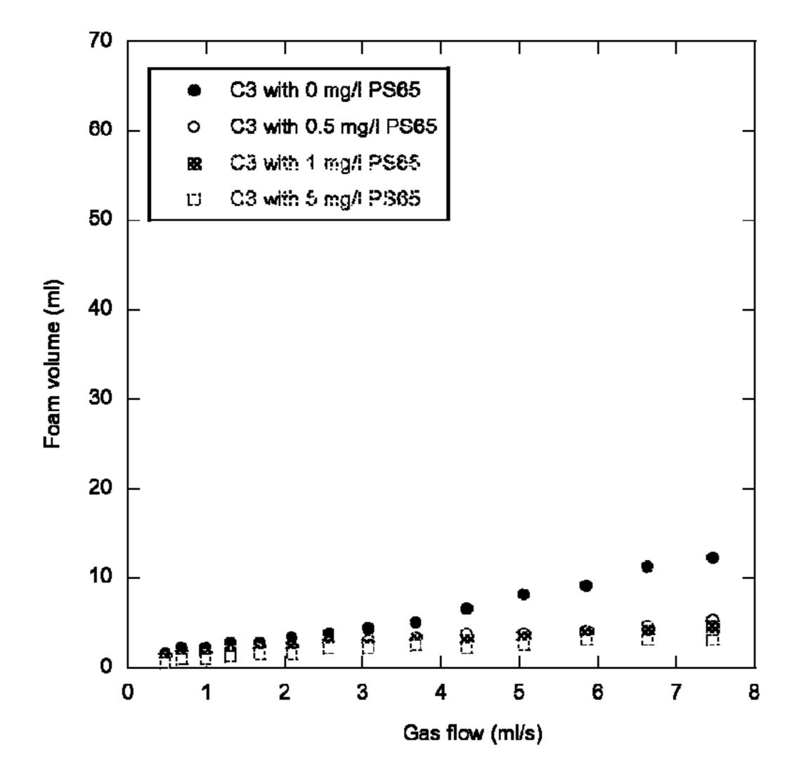
Figure 9: Bikerman foaming test with C3 and 0-5 mg/l PS65.
