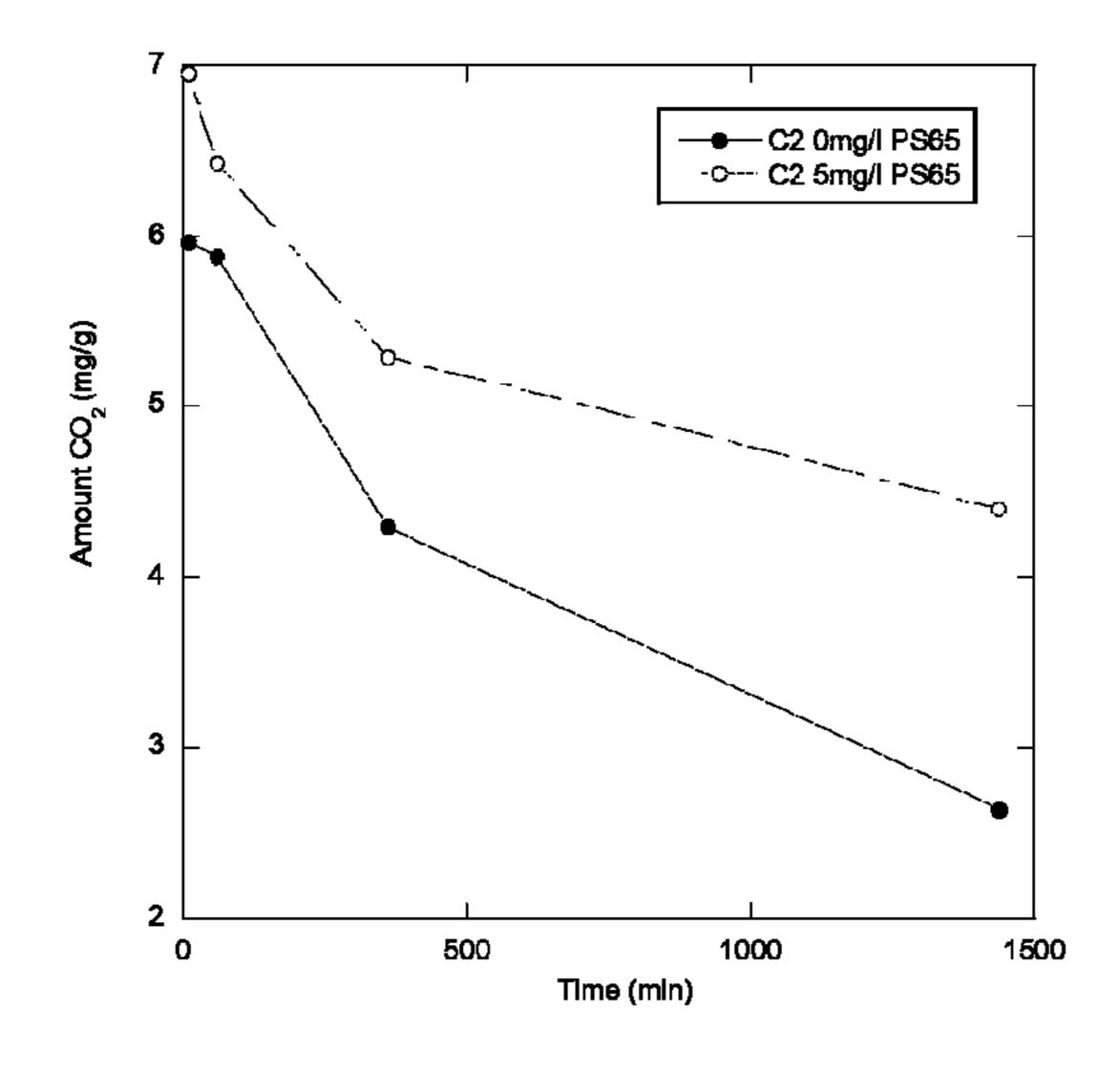
Figure 10: Amount of CO<sub>2</sub> (in mg/l) retained for C2 after removing the cap from the bottle.
