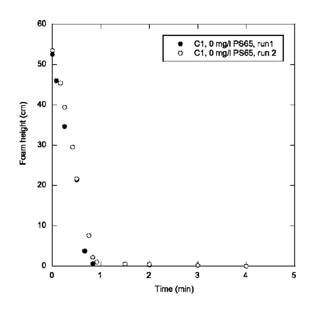
Ross Miles test for C1 with 0 mg/l PS65, run 1 and run 2.
