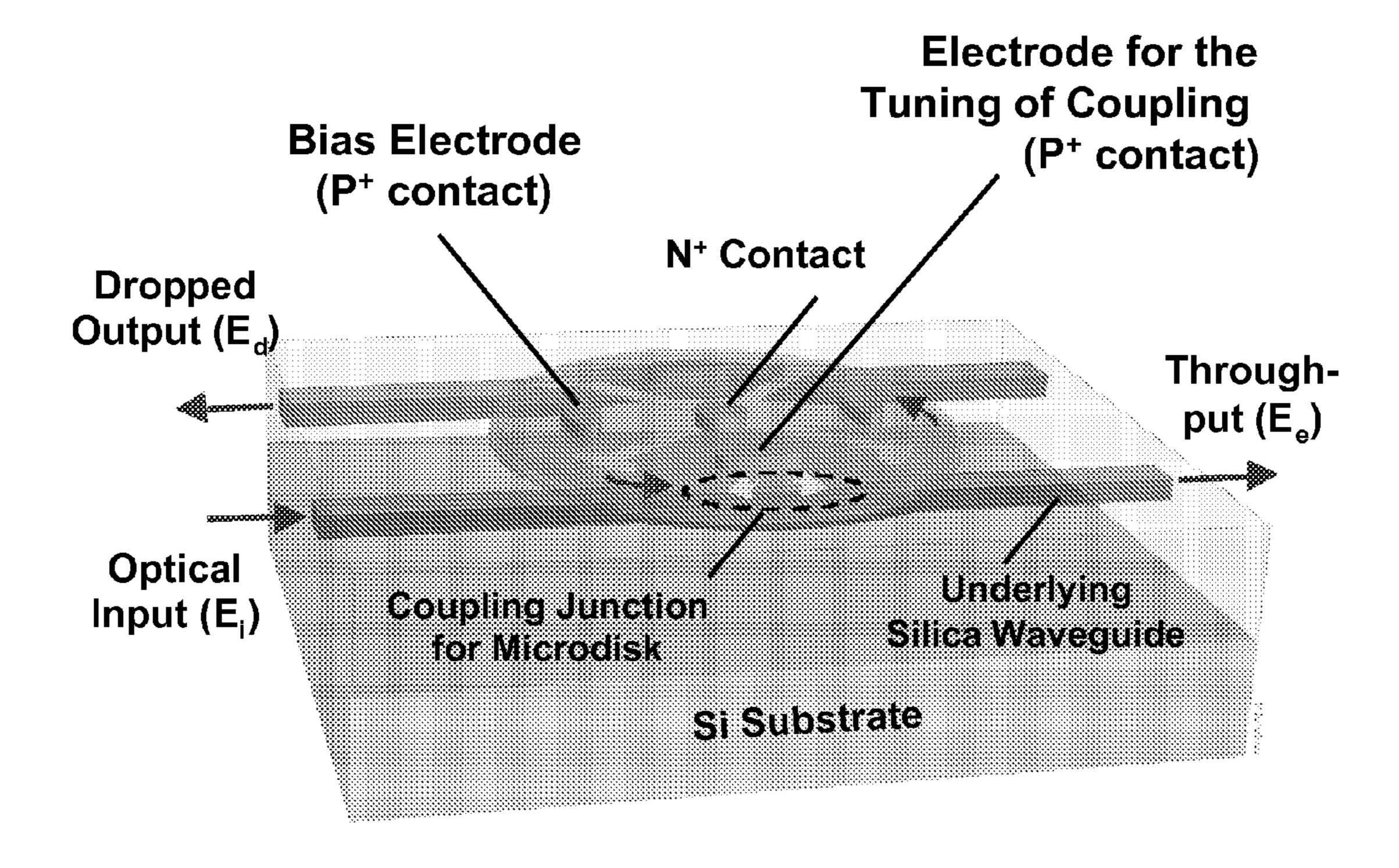
Heterogeneously Integrated Si Microdisk: **Electrode** Bias Optical Input Dropped next Unit Cell same row Outpu Cell
