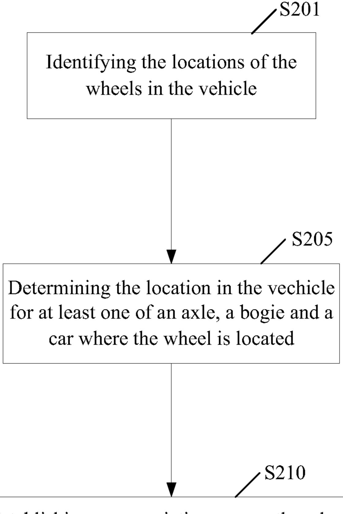
Establishing an association among the wheel inspection data, the locations of the wheels and the location of at least one of the axle, the bogie and the car where the wheel is located
