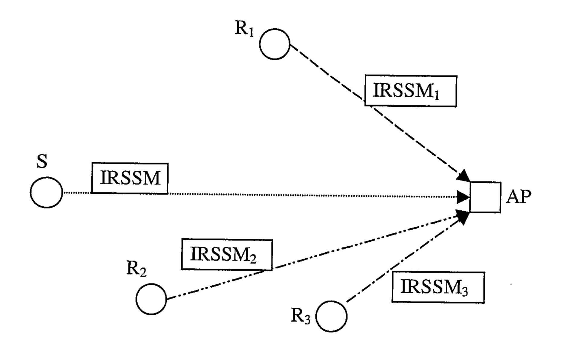
Figure 1 Stations send IRSSM frames to AP at different times
