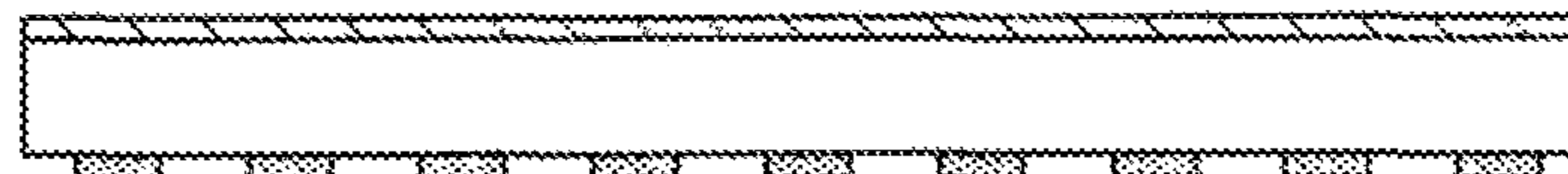
2. Ti/Cu SEED LAYER DEPOSITION BY PVD
