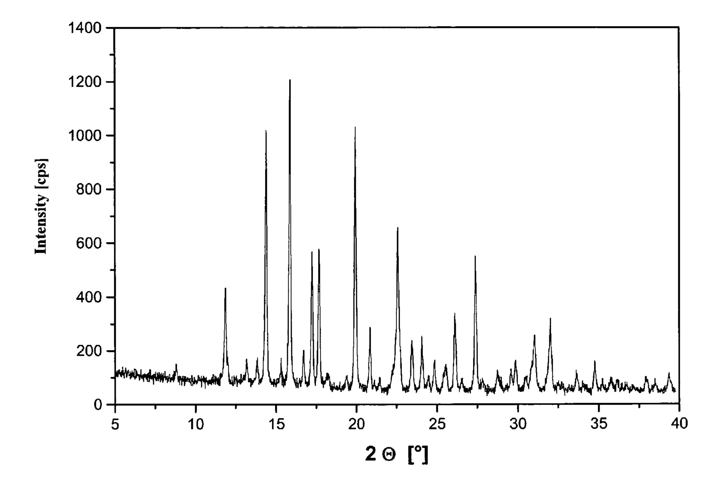
Figure 2: X-ray powder diagram of anhydrous tiotropium iodide
