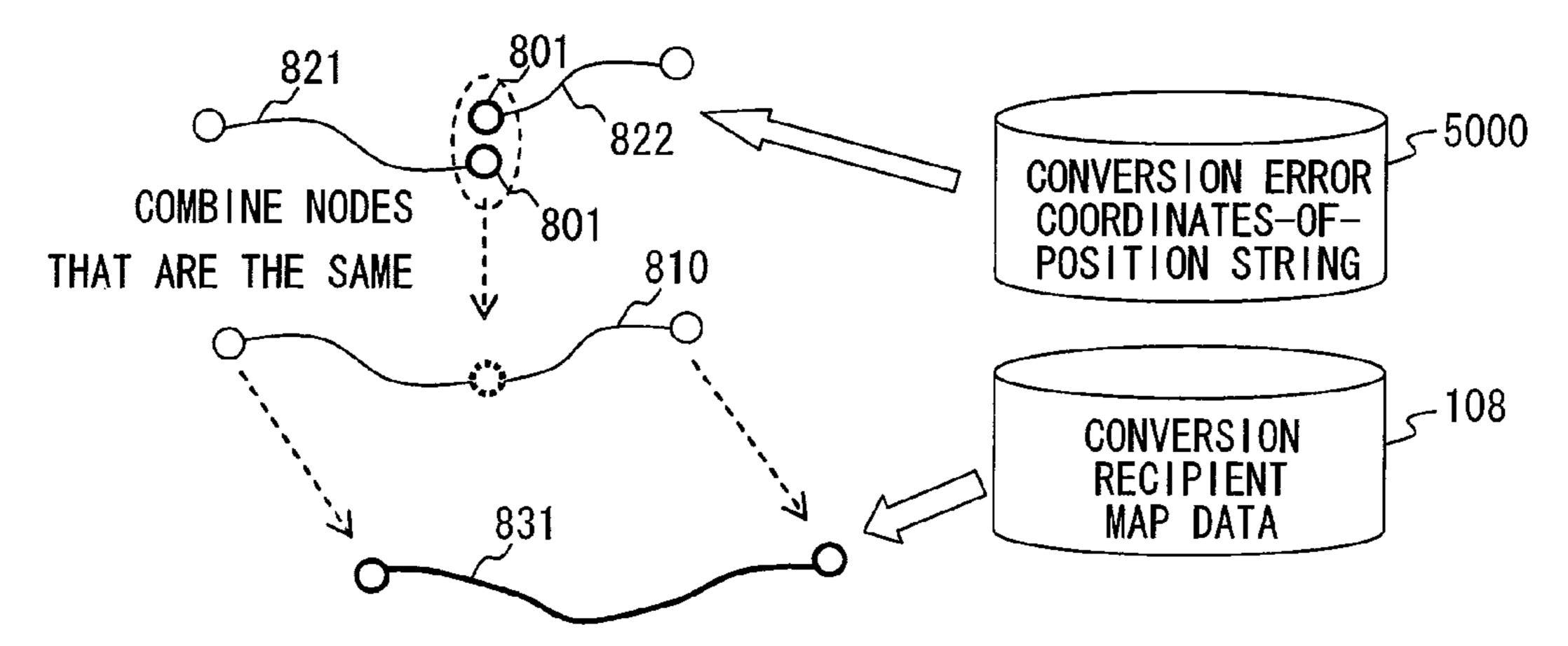
SPECIFY CORRESPONDING NODES BY MATCHING PROCESSING TO CONVERSION RECIPIENT NODE, AND SPECIFY ROAD SECTION USING ROUTE SEARCHING
