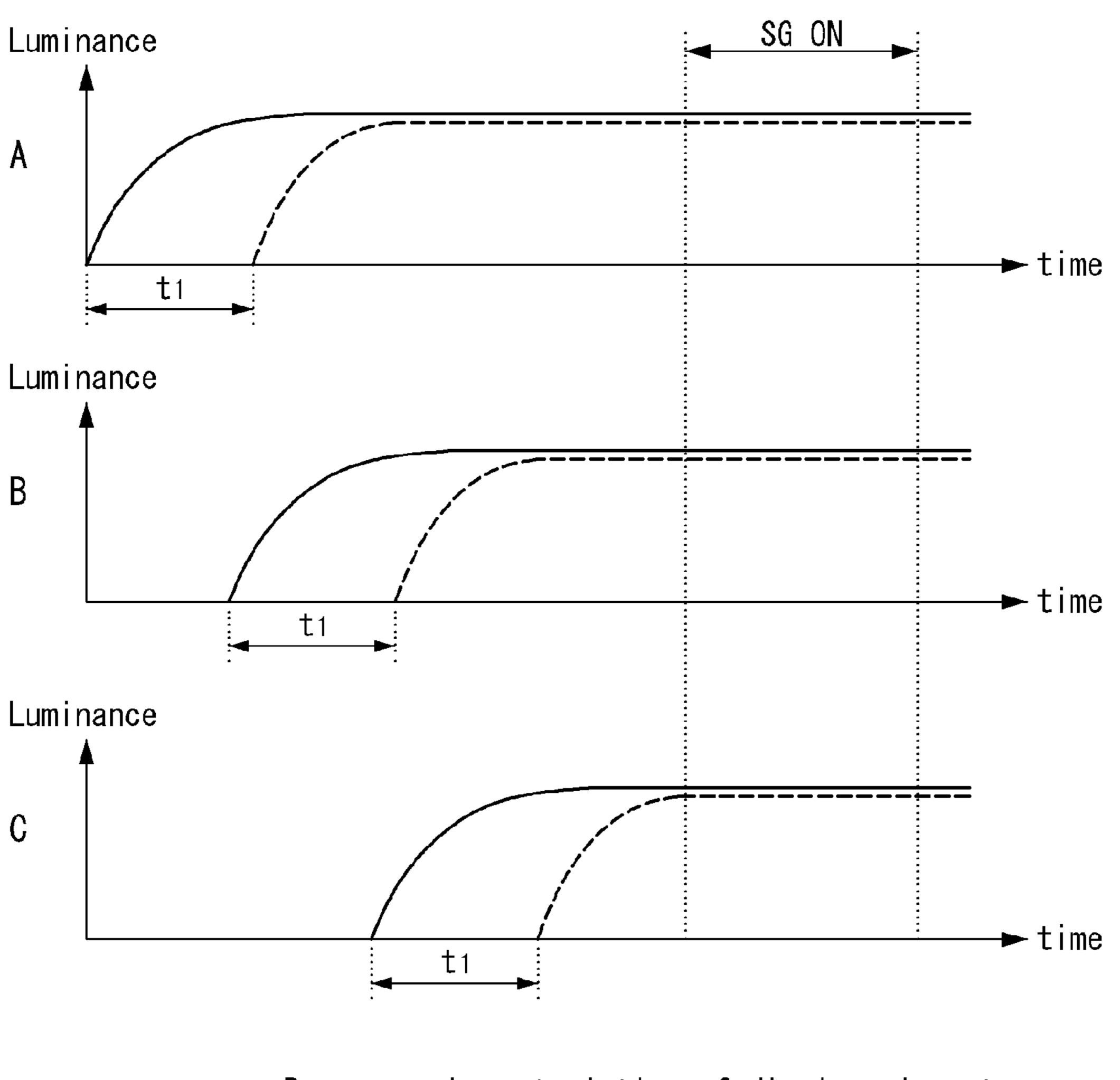
Response characteristics of display element ---- Response characteristics of active retarder cell (AR)
