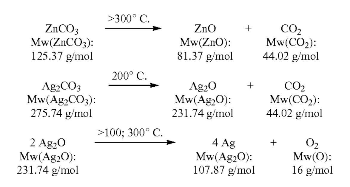
Process control by TGA (20° C./min): three peaks of mass loss are found: 155° C.; 237° C.; 350° C. Process control by DSC (20° C./min): two peaks of thermal activity: 170° C. (-26 J/g); 248° C. (191 J/g)
