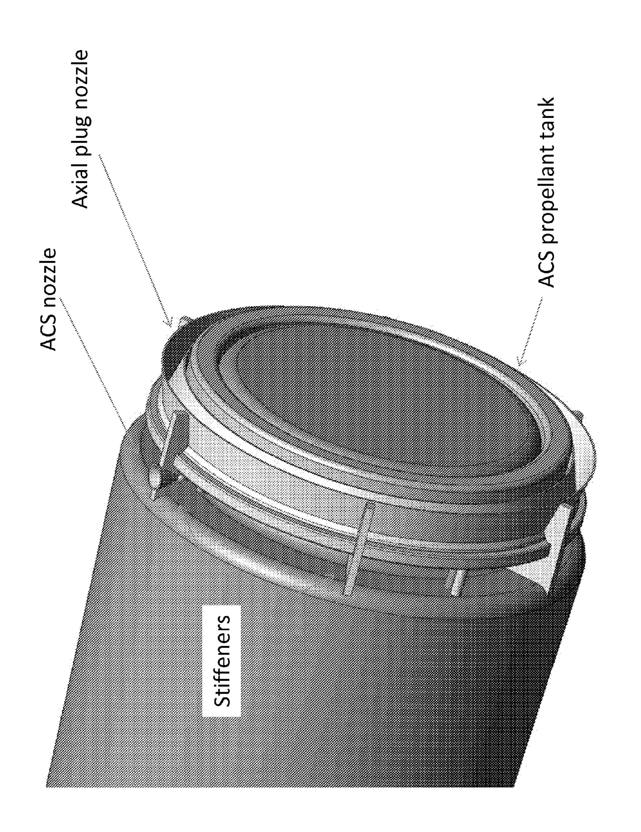
Figure 4. Rocket nozzle and Attitude Control System (ACS)
