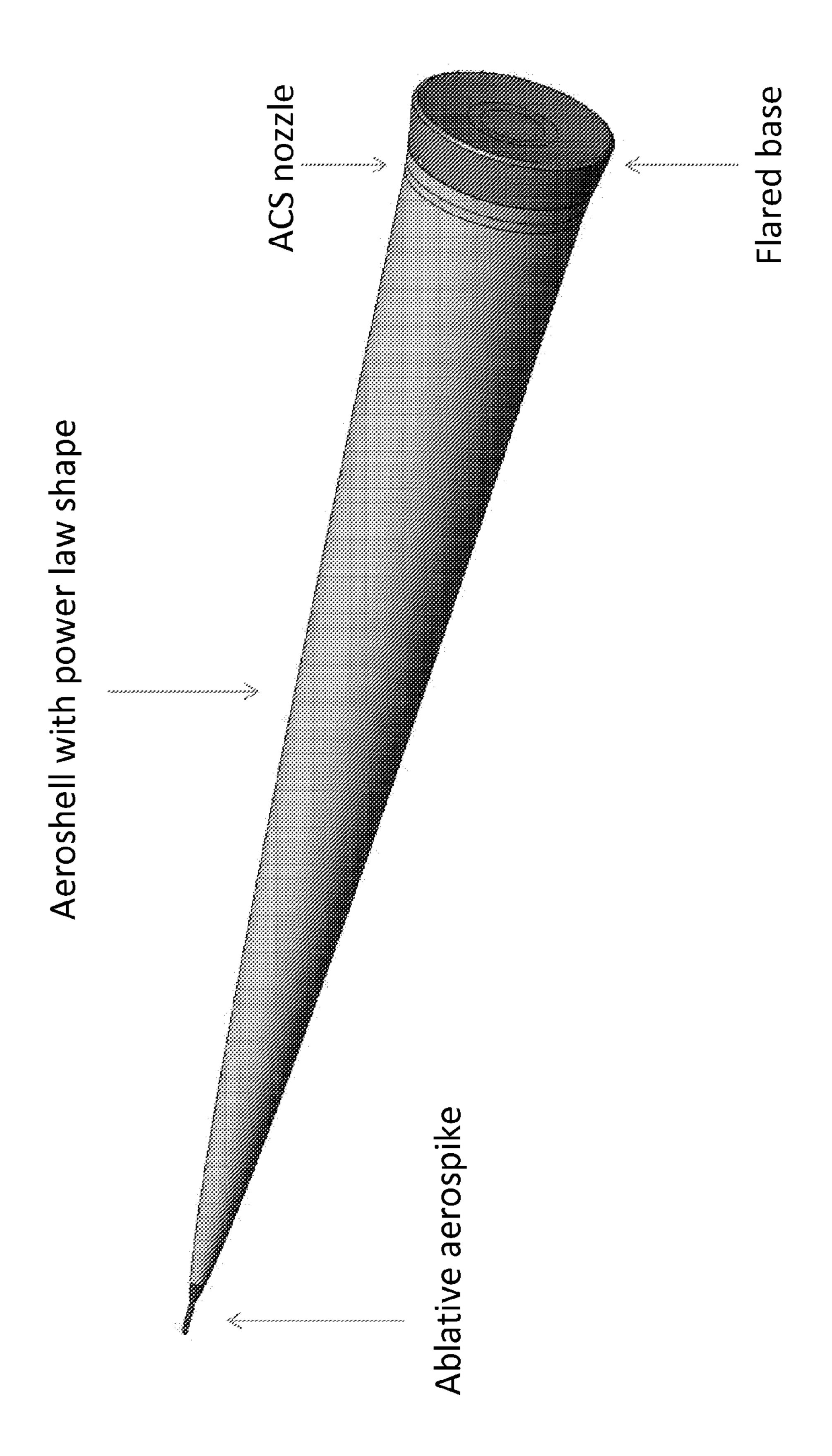
Figure 2. Vehicle aero-shell
