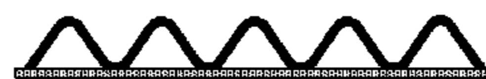
(c) Single plate-wave combination structure
