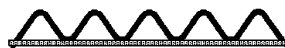
(c) Single plate-wave combination structure
