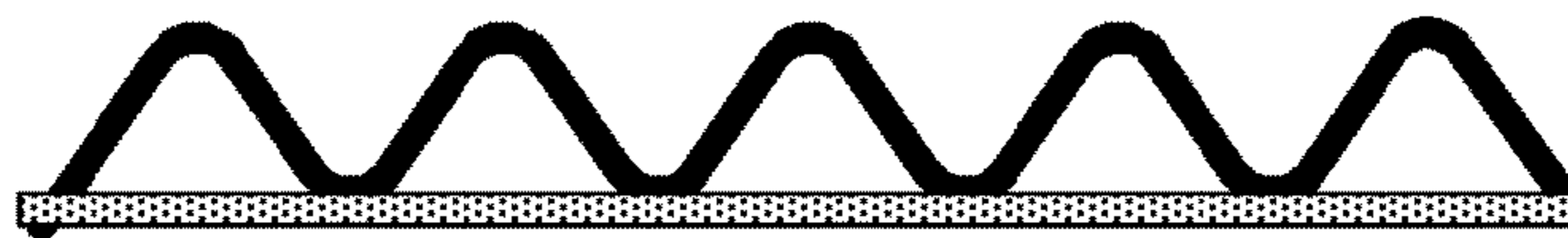
(c) Single plate-wave combination structure
