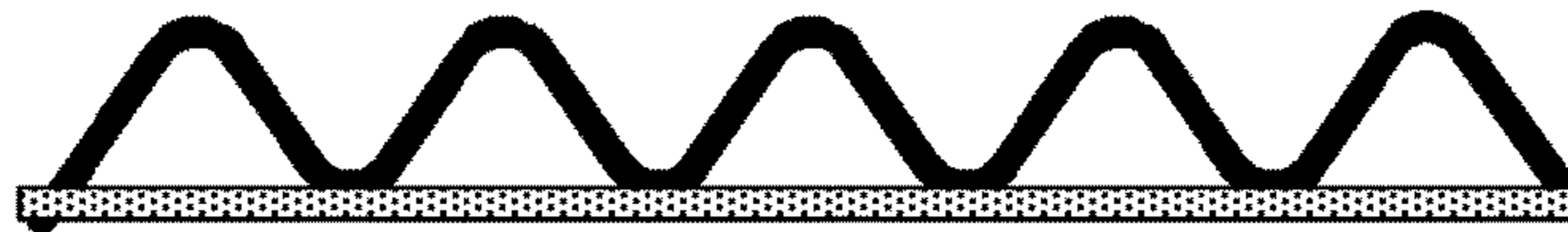
(c) Single plate-wave combination structure
