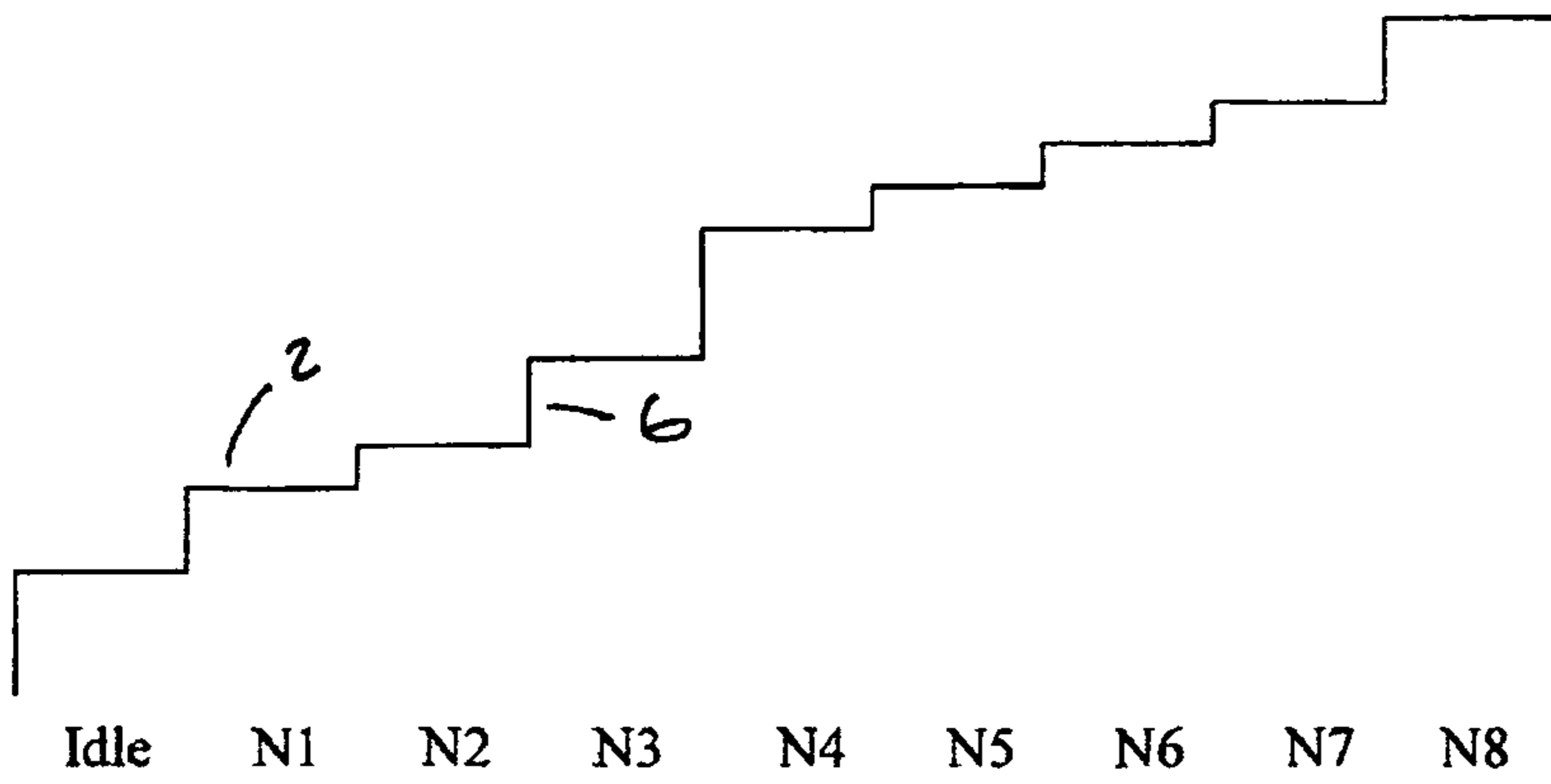
Figure 3: Plunger's Timing surfaces for all Notch Positions (horizontal surfaces are located every 25 degrees from either starting position)
