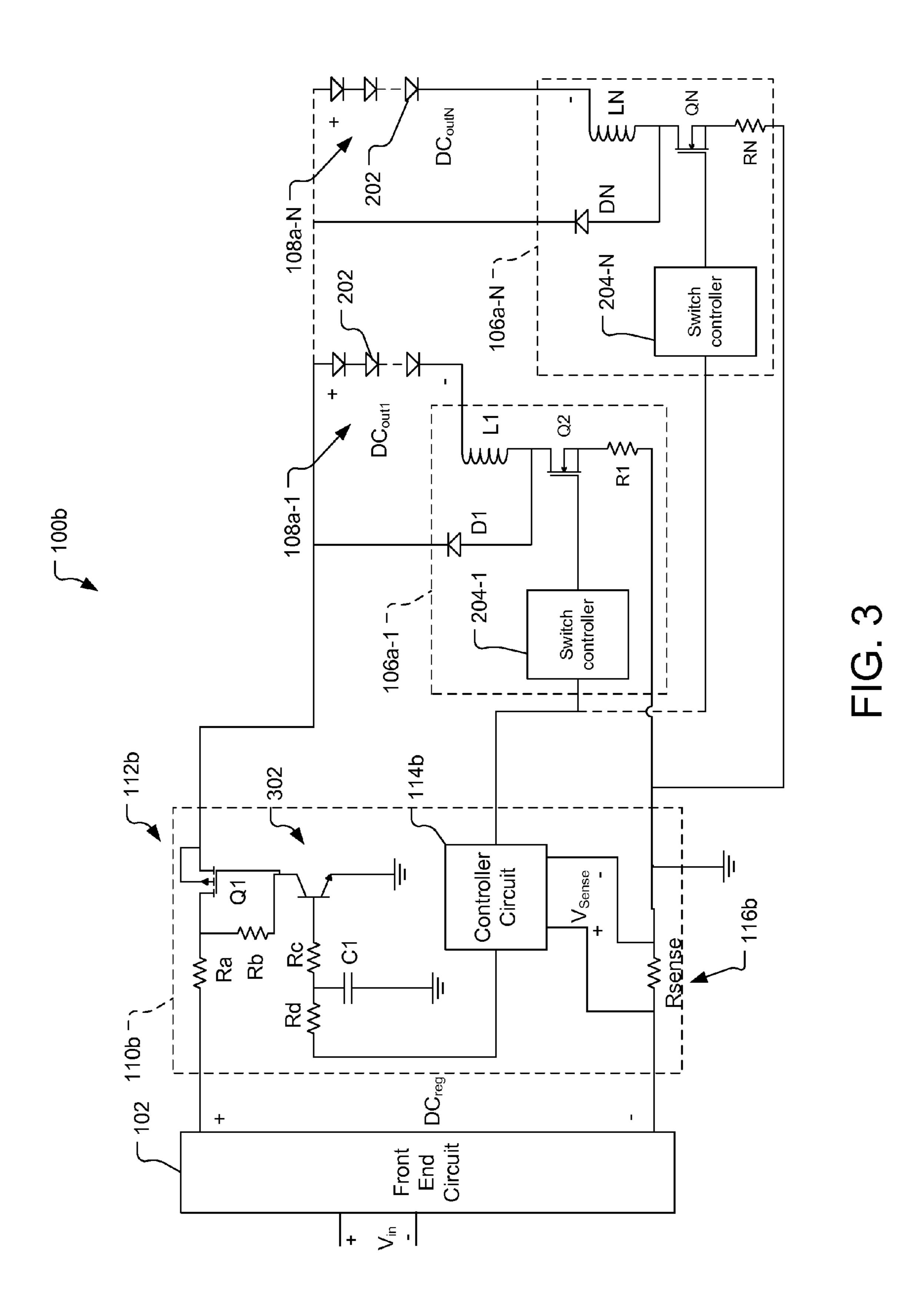
400 PROTECT AGAINST SUPPLYING EXCESSIVE POWER AT ONE OR MORE OUTPUT CHANNELS OF A MULTIPLE OUTPUT CHANNEL POWER SUPPLY
