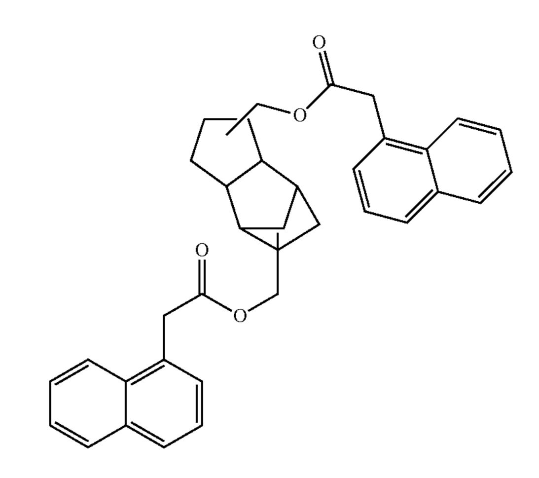
Molecular weight 532 g/mol Refractive indices at 20° C.:  $n_g$  (435.8 nm)=1.6407  $n_F$ ' (480.0 nm)=1.6282  $n_e$  (546.1 nm)=1.6159  $n_D$  (589.3 nm)=1.6102  $n_{C'}$  (643.8 nm)=1.6050 Abbe number (dispersion):  $V_e$ =26.5
