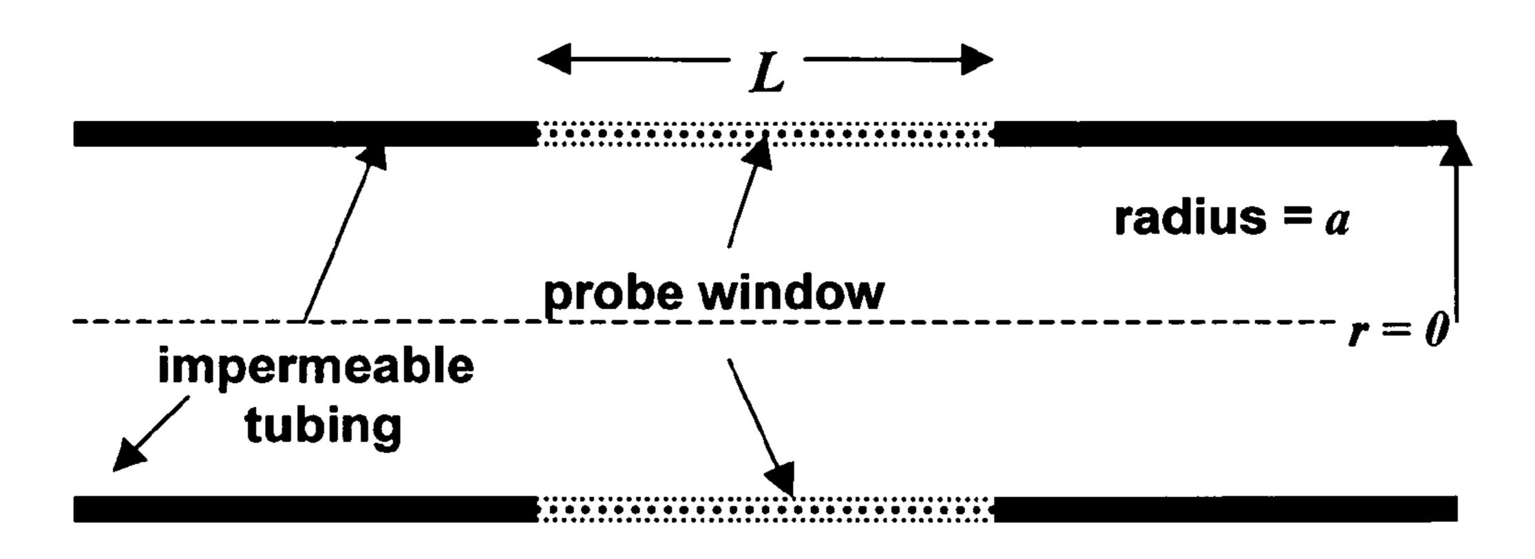
Figure 1. Schematic diagram of microdialysis probe. (Prior art)
