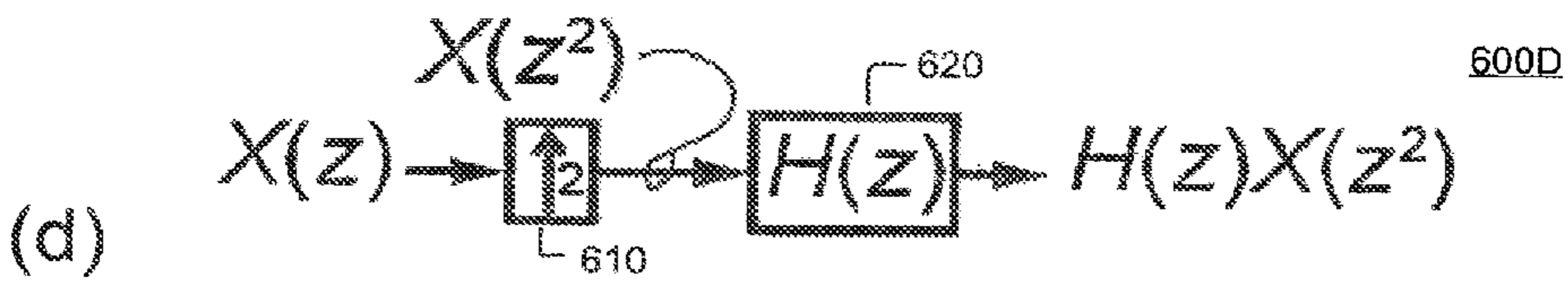
Fig. 6. Halfband filter and up-sampler. (a) Up-sampler mathematics. (b) Up-sampler operation. (c) Halfband anti-imaging filter. (d) Mathematical relations for up-sampler system.
