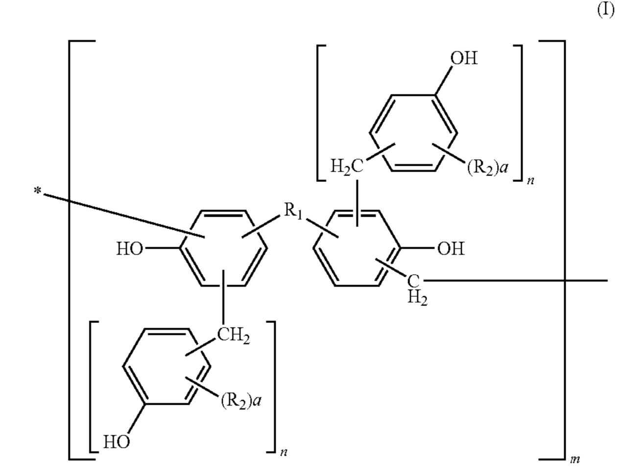
wherein R<sub>1</sub> represents either one of a hydrocarbon radical of 1 to 11 carbon atoms, a SO<sub>2</sub> group, an oxygen atom and sulfur atom, R<sub>2</sub> represents a hydrocarbon radical of 1 to 11 carbon atoms, "a" represents an integer of 0 to 3, "n" represents an integer of 1 to 2, and "m" represents an integer of 1 to 10.
