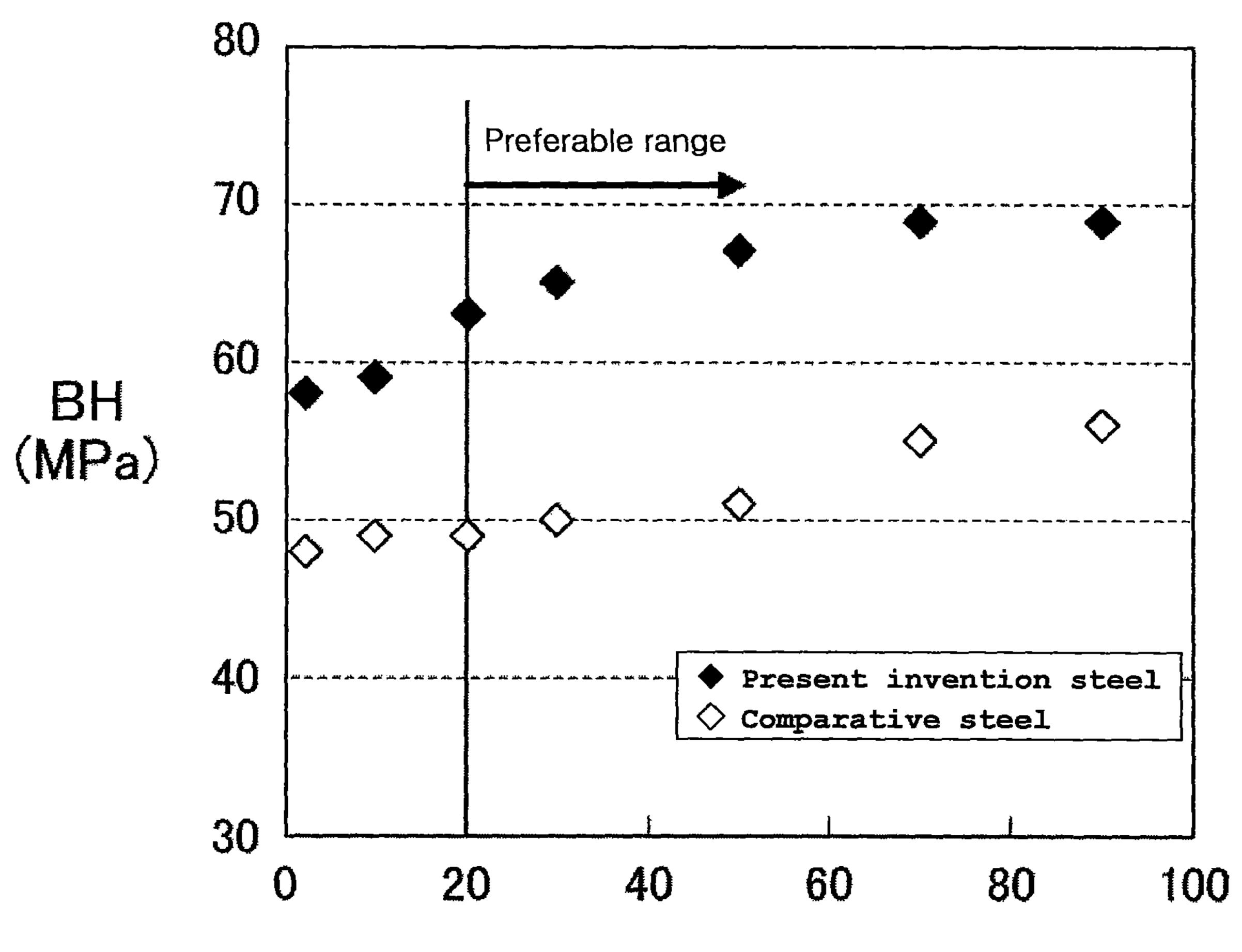
Cooling rate up to 640°C after rolling (°C/s)
