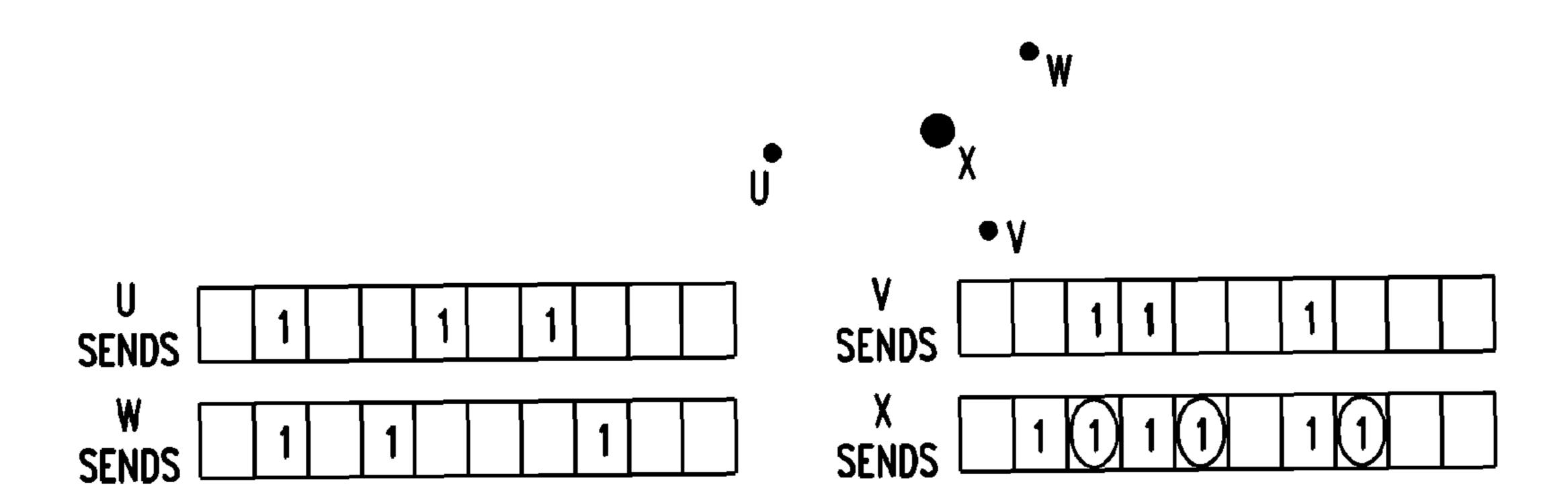
THE CIRCLED SLOTS ARE THE UNIQUE SLOTS IN WHICH ONLY ONE NODE TRANSMITS, THOUGH CH & DOES NOT KNOW THAT
