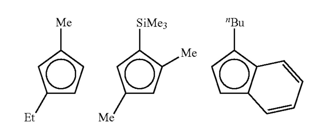
If the uncoordinated Cp does not contain a two-fold axis or perpendicular mirror plane, and the  $R^A$  substituents do possess chirality of their own, the faces are diastereotopic. The Cp is prochiral in this case as well, and its coordination to a metal results in two diastereomers (i.e., not mirror images of one another).
