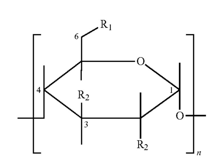
The CD's internal cavity size (i.e.,  $\alpha$ ,  $\beta$ ,  $\gamma$ ) can be considered and the functional group modification can be suitable for changing the desired bulk polymer and surface polymer characteristics in addition to forming an inclusion complex with targeted volatiles or impurities. To achieve a specific result, more than one cavity size and functional group may be necessary.
