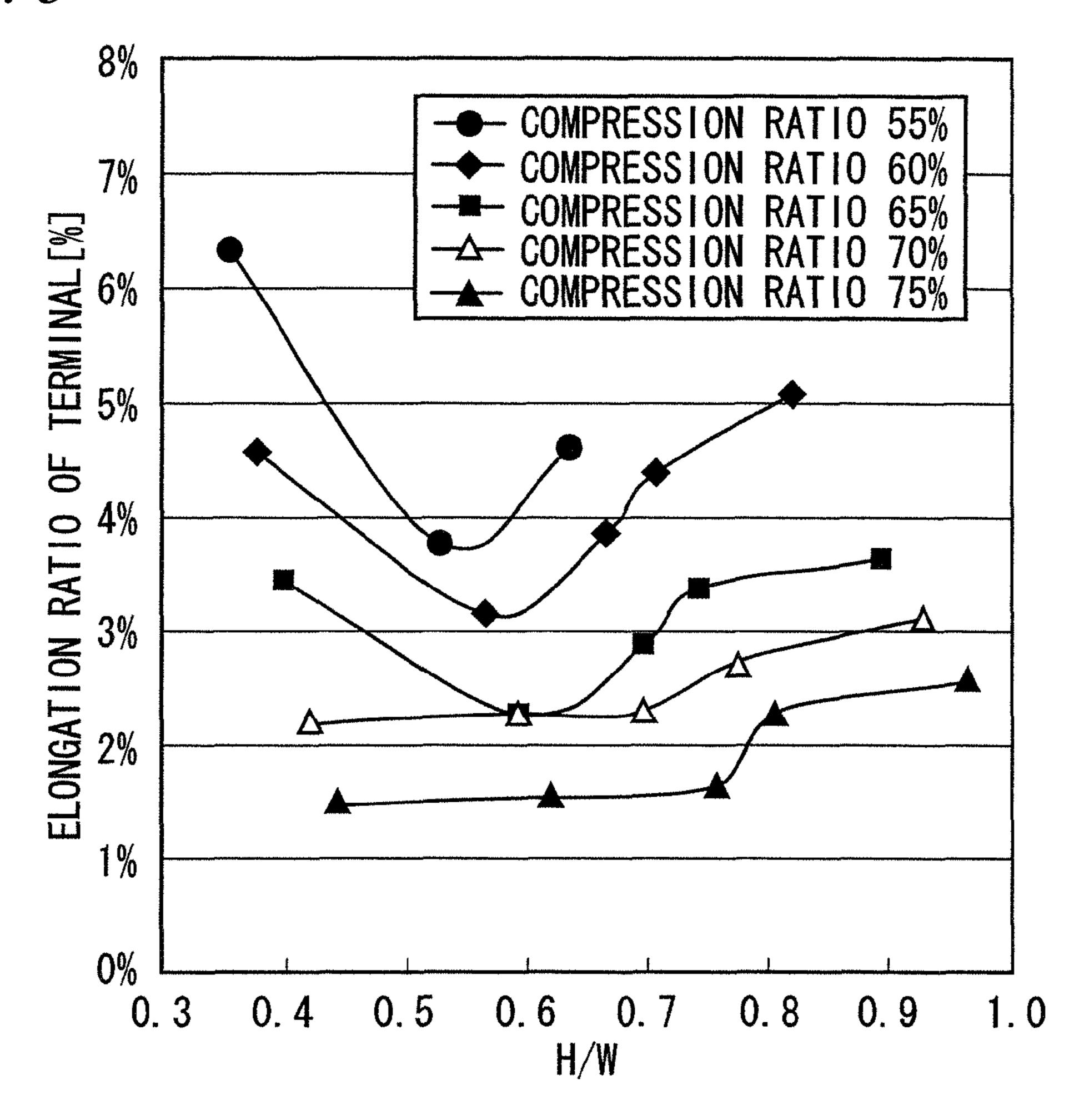
TERMINAL MATERIAL: CAC 60 SHEET THICKNESS: 0. 25 mm
