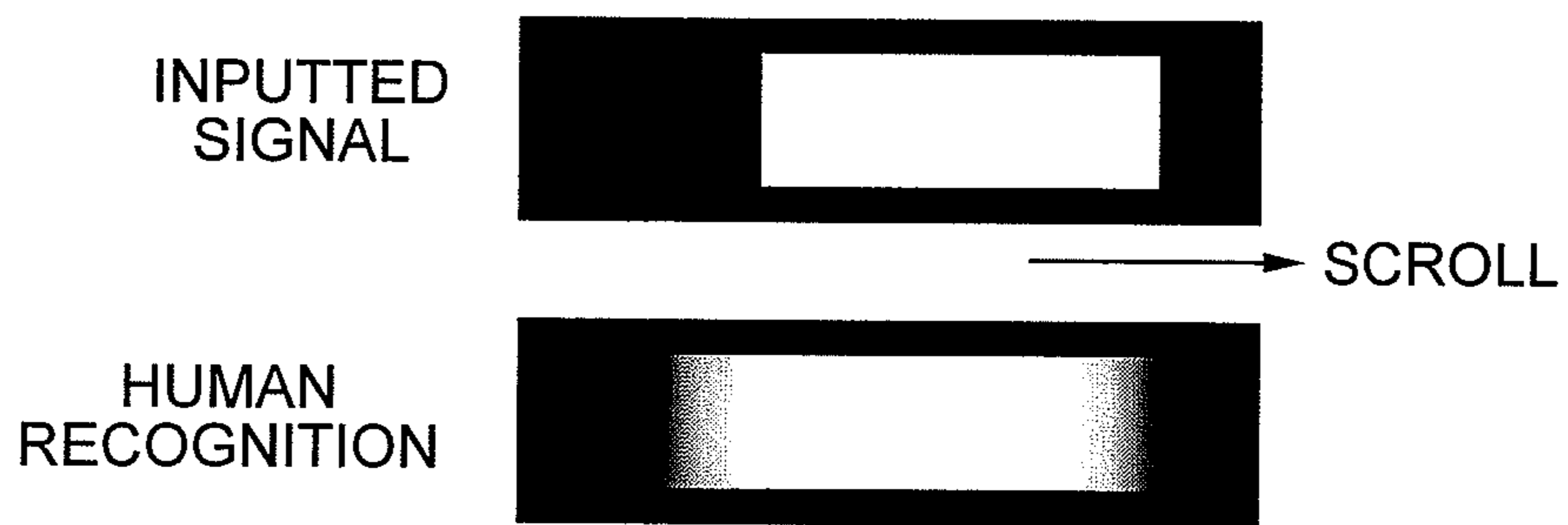
TAILING CAUSED BY BLACKENING
