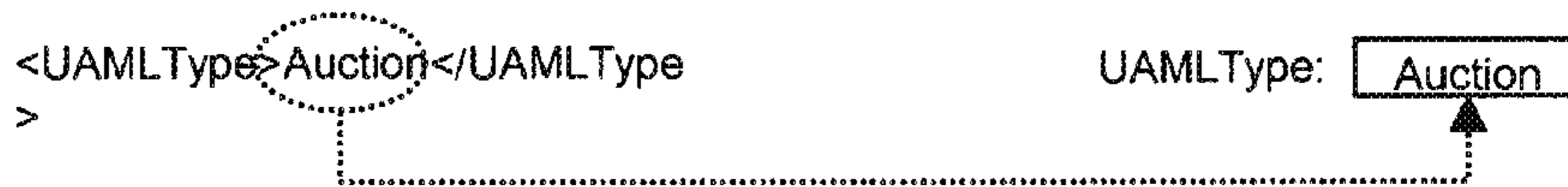
FIG. 15 UAML Subsystem: Parsing and Mapping of UAML Data in User's Web Page to UET Company Database Record
