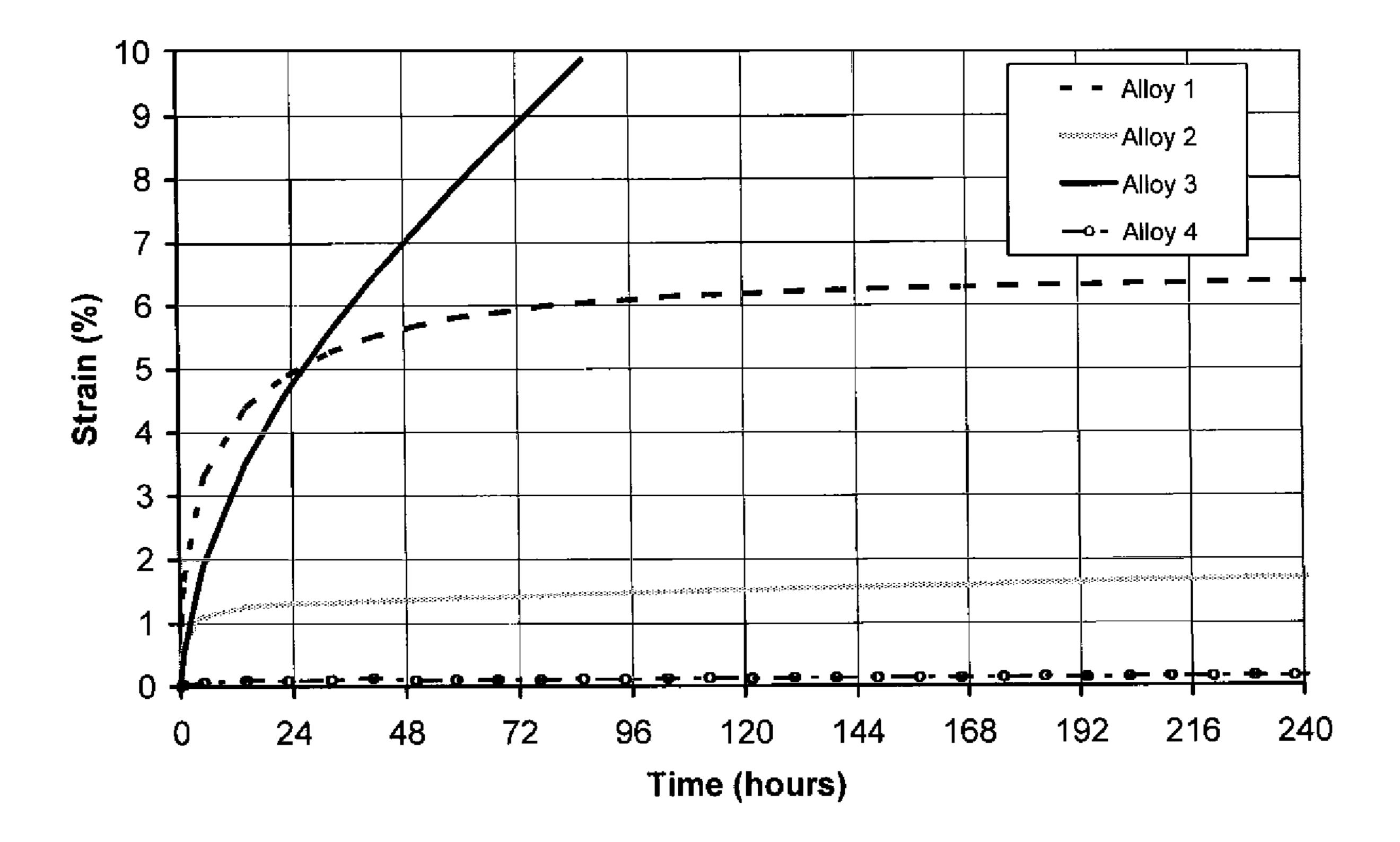
Strain development during creep test.
