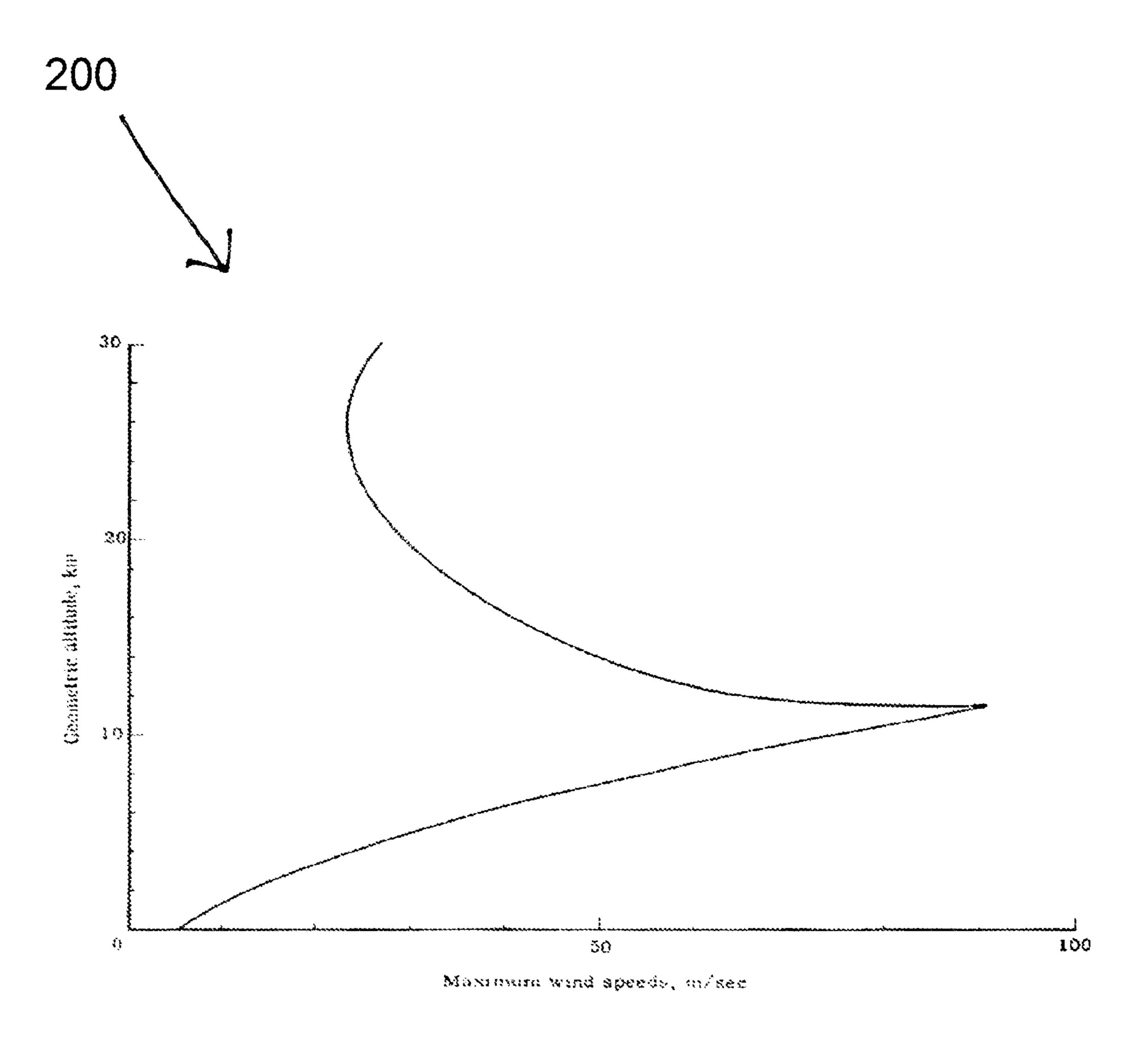
Graph 1: A Typical Statistical Maximum Wind Speed Curve
