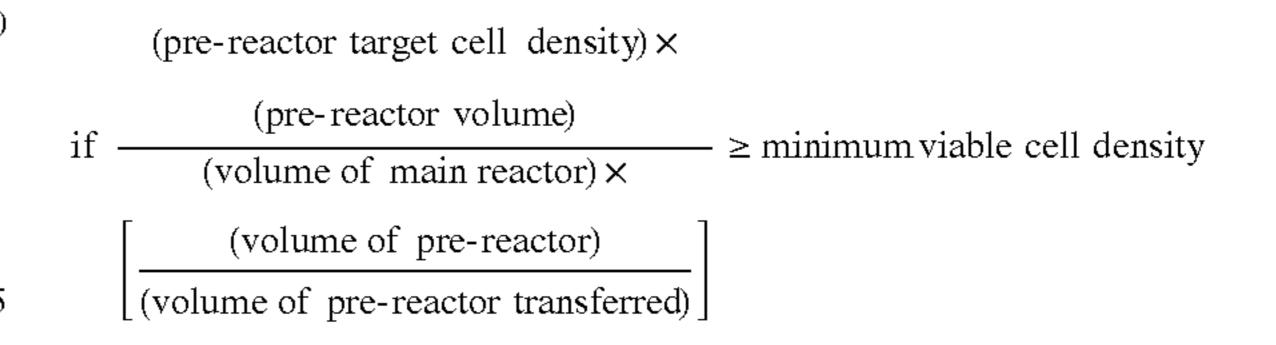
then a volume of the pre-reactor is transferred to a main reactor in an amount effective for providing a minimum cell density in the main reactor; or
