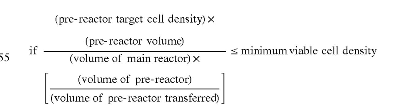
then a volume of the main reactor may be adjusted and a volume of the pre-reactor may be transferred in an amount to provide a minimum viable cell density in the main reactor. The volume of the main reactor is then increased over time to a desired volume while maintaining a minimum viable cell density.
